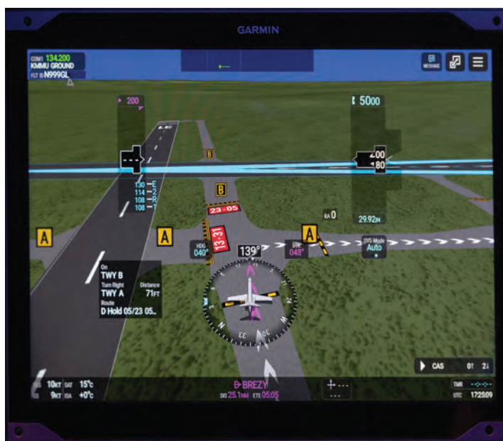
With taxiway routing, G3000 Prime can automatically select the route to a selected airport destination.
