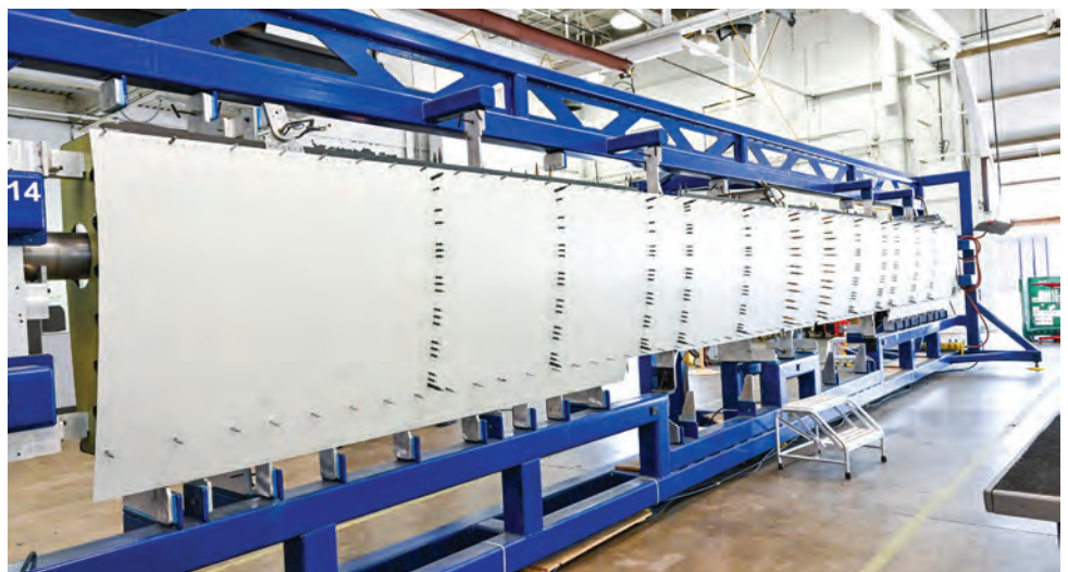
This 35-foot wing component is the largest composite part that the company has ever made.
