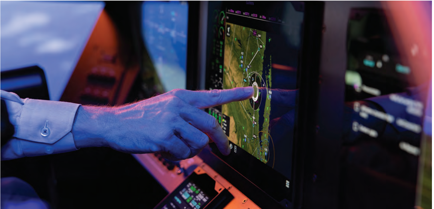
The radial menu is a new feature for G3000 Prime, making flight plan changes and information access just a touch away.
