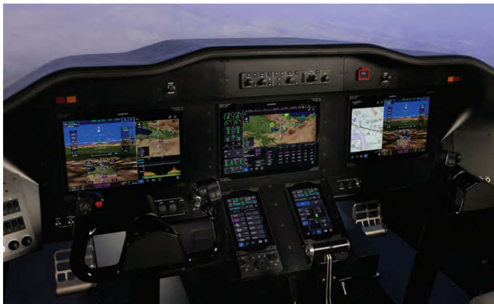
A typical G3000 Prime cockpit in a Part 23 jet will look like this, with a total of five touchscreens.
