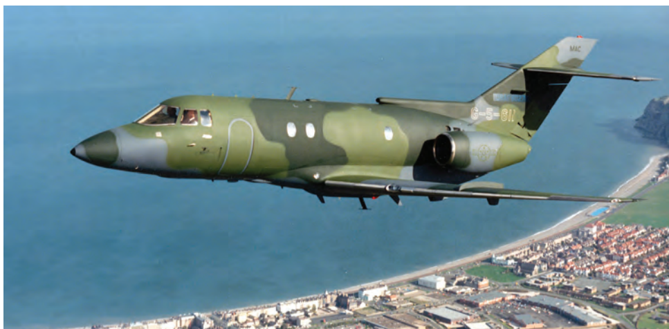
Six 125-800s were outfitted by LTV Sierra for service with the U.S. Air Force as navigation and landing aid checkers. They served for just over a year before going to the FAA.
