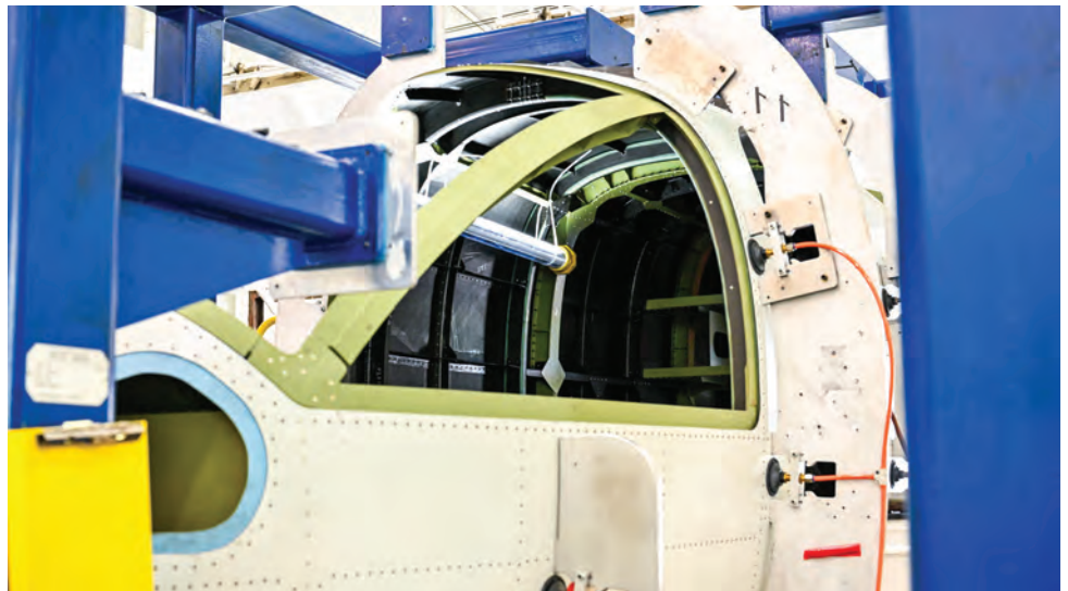
The composite Nexus forward fuselage and aluminum windshield framing.
