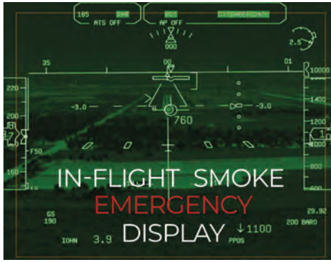
SAVED integrates a head-up display into a full-face oxygen mask for in-flight smoke emergencies.
