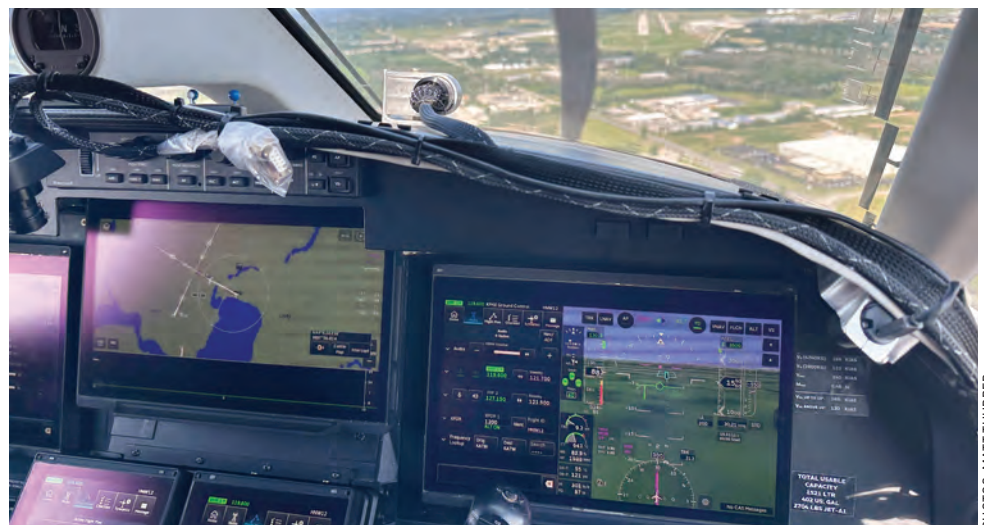
The Anthem integrated avionics system aims for an intuitive touchscreen display interface.
