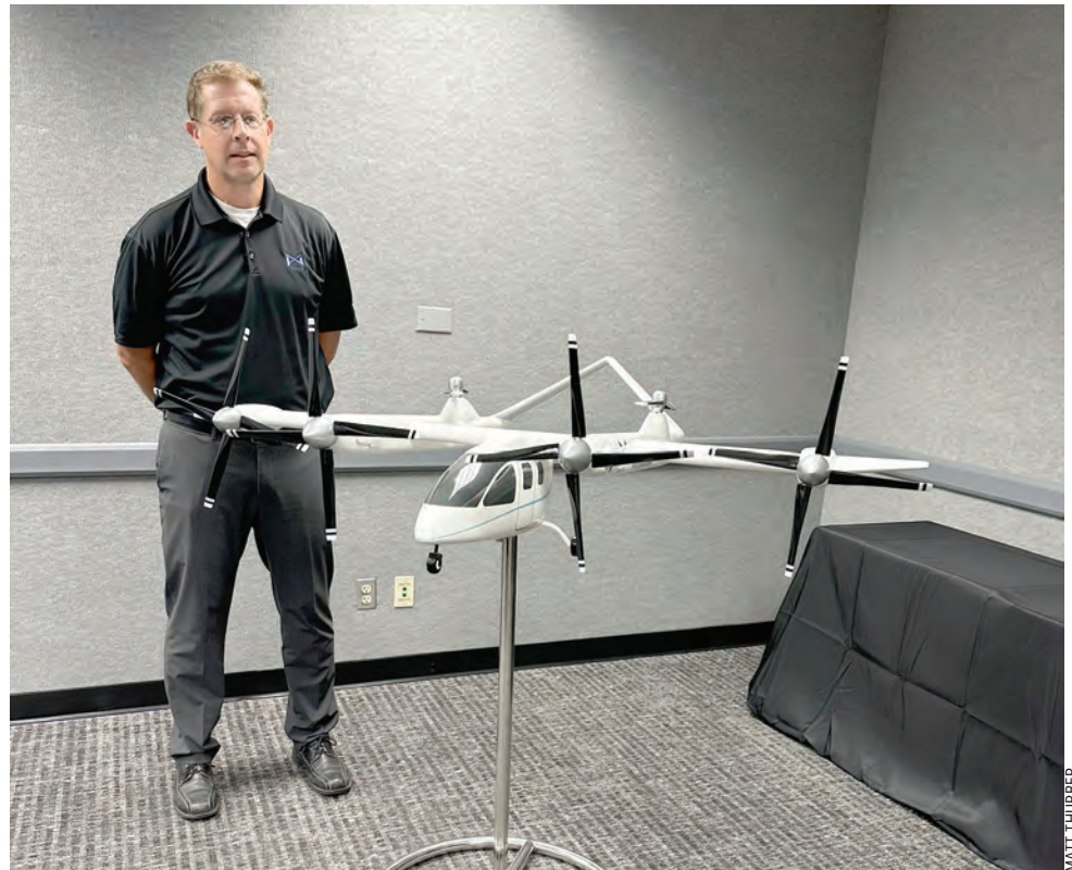
Textron eAviation director of engineering JD Terry with a model of the Nexus eVTOL aircraft. All four tilting propulsion units are shown in the forward-tilt position.
