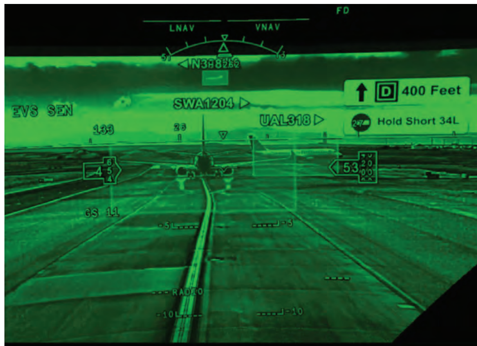
The air traffic controller's instructions are shown on the top right in this enhanced vision system head-up display image, along with highlighting the proper route over the ground.
