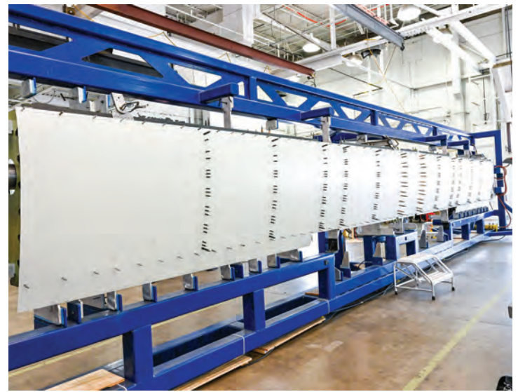
This 35-foot wing component for the Nexus eVTOL aircraft is the largest composite part that the company has ever made.
