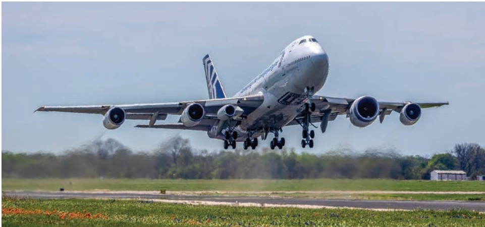
Rolls-Royce conducted flight trials of its Pearl 10X on the company's 747-200 testbed in Tucson, Arizona.
