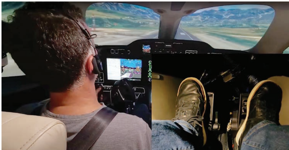
Proper de-crabbing and brake use can be observed in the HondaJet simulator.
