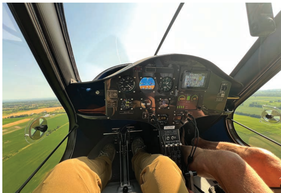
Flying the Velis Electro means learning a new power-management technique by monitoring power output, state of charge, and time remaining at the various power settings.
