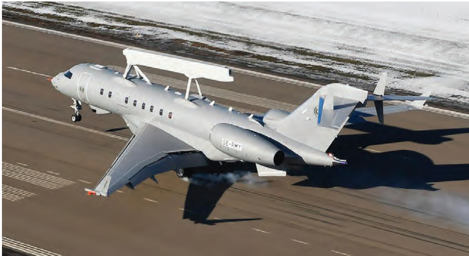
Based on the Bombardier Global 6500, Saab's GlobalEye offers range of up to 12,223 km and endurance of more than 18 hours. Customers include the UAE, Sweden, and France.
