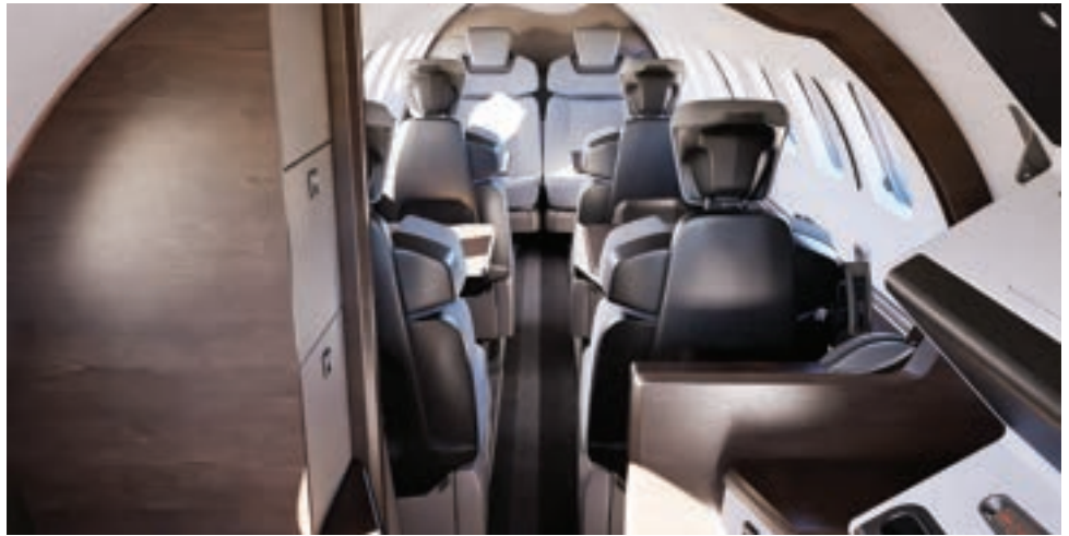
SyberJet engineers have gained 1 to 3 inches more cabin width in the SJ36 redesign.
