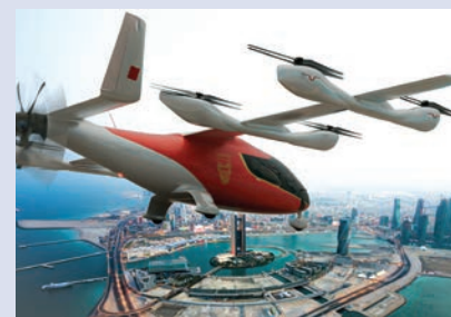
Eve believes its 'lift and cruise' design minimizes dust and sand exposure.
