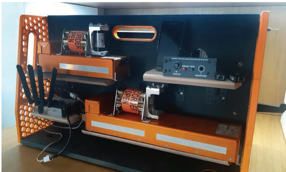
Flight Data can be streamed in near real-time via satellite from Honeywell’s Connected Recorder system, which forms the backbone of its Black Box in the Sky initiative.
