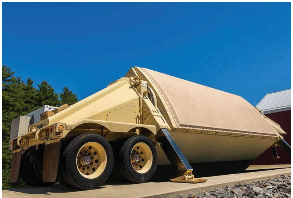
The TPY-2 long-range air defense radar supports the THAAD theater-defense missile system.
