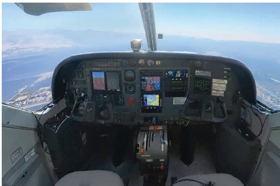
Reliable Robotics has flown dozens of unpiloted flights in this modified Cessna Caravan.
