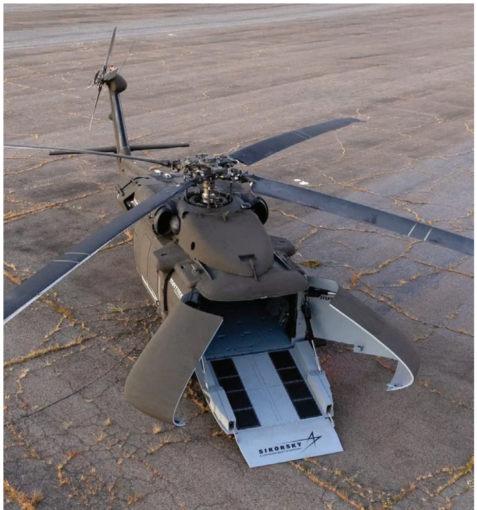
With no need for a cockpit, the U-Hawk features doors and a ramp for loading vehicles.
