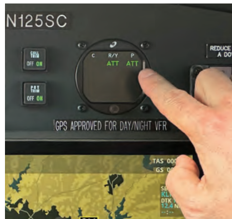
The AStar installation uses a Mid-Continent Flex instrument as the mode annunciator.
