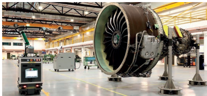
Pratt's Eagle Services Asia facility here in Singapore (left) is pioneering automation to reduce process times for engine inspections and assembly. Atlas (below) uses a robotic arm to stack low-pressure compressor sections.
