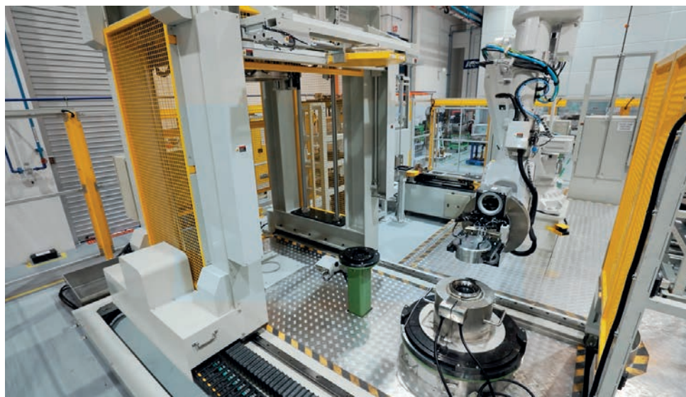
Pratt's Eagle Services Asia facility here in Singapore (left) is pioneering automation to reduce process times for engine inspections and assembly. Atlas (below) uses a robotic arm to stack low-pressure compressor sections.
