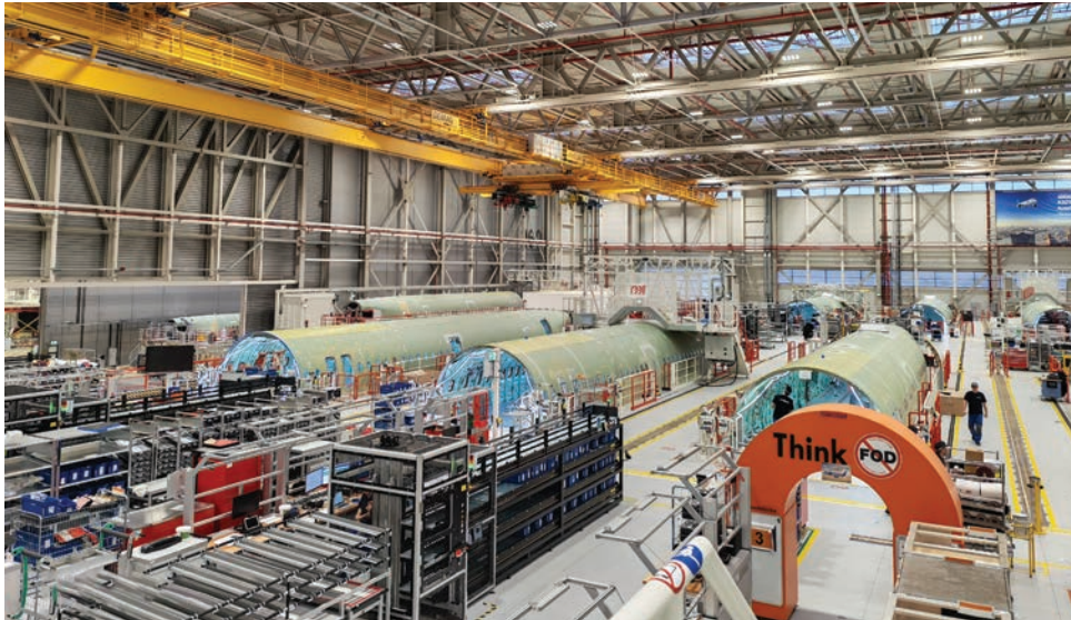
Green A321XLR fuselage sections await connection to forward fuselages at the Airbus Hamburg facility.
