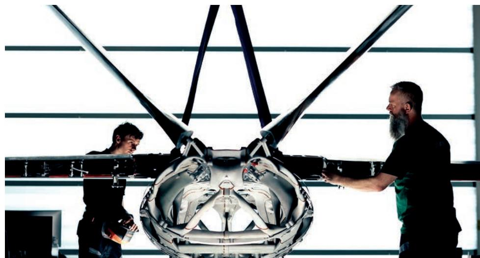
The 3D-printed fuselage for Saab's autonomous air vehicle includes topology-optimized complex shapes and varying thicknesses to find the best structural load paths and reduce parts counts.
