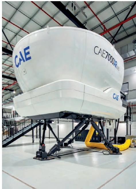
CAE's 7000XR full-flight simulator for the Boeing 777X features a 3D visual system with photorealistic imagery under all types of weather conditions, and enhanced moving models.
