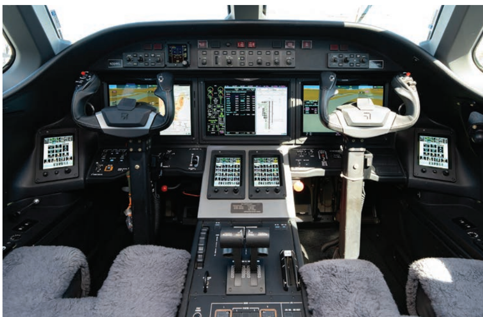
Switching to the Garmin G5000 avionics suite made for an uncluttered and welcoming flight deck.
