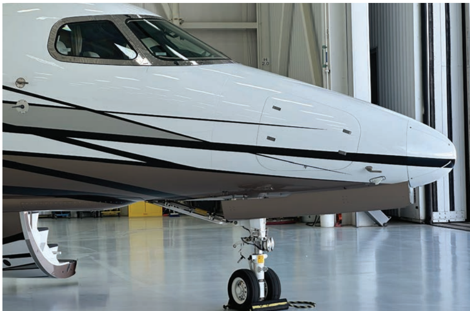
Electrically heated windshields and a new nose design set the Ascend apart from the XLS.
