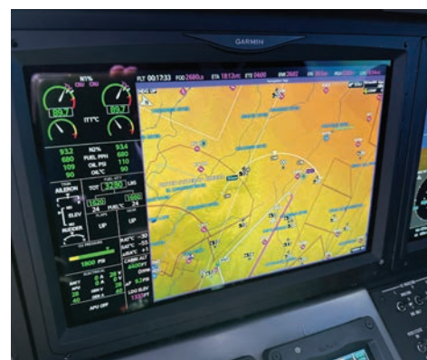
Cruising at FL360, the Ascend's PW545D engines each burned 680 pph.
