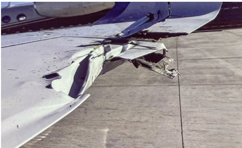
A forklift driver, previously suspended for reckless driving, subsequently damaged this Gulfstream.
