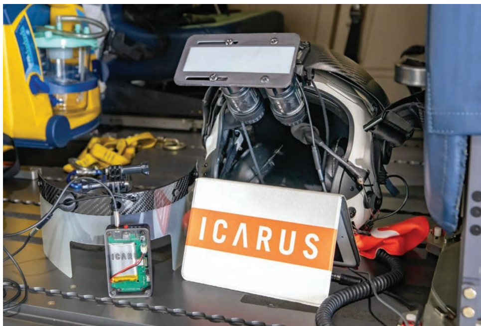
The Icarus Smart View Limiting Device is also available in a night-vision goggle-compatible panel, so pilots can practice inadvertent IMC encounters at night while wearing goggles.
