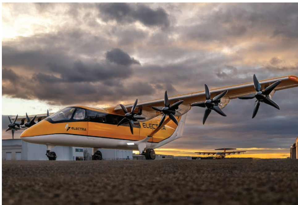
Electra's hybrid-electric, nine-passenger EL9 hybrid takes off and lands in just 150 feet.
