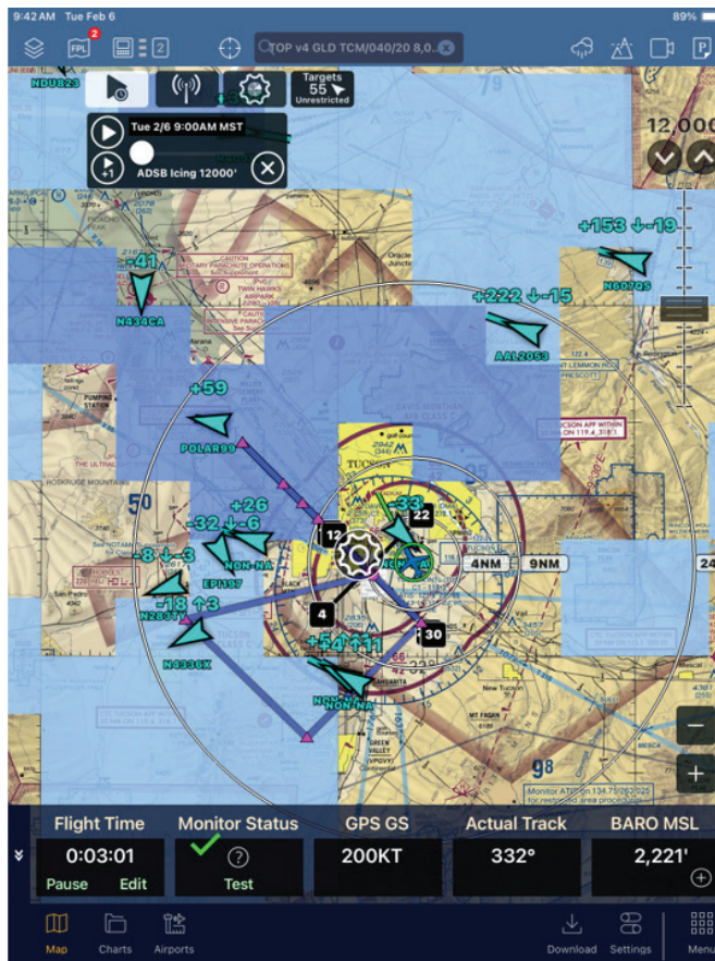
The Universal Avionics FlightPartner electronic flight bag can display fused TCAS/ACAS and ADS-B In traffic.
