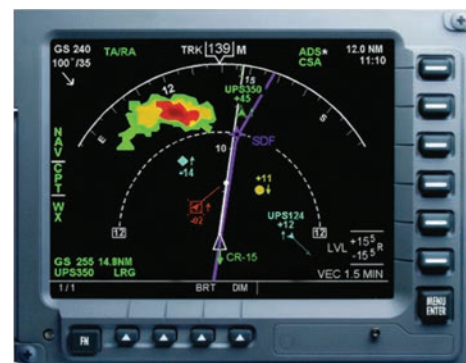
FreeFlight Systems RANGR-IQ ADS-B system can include TCAS II integration.
