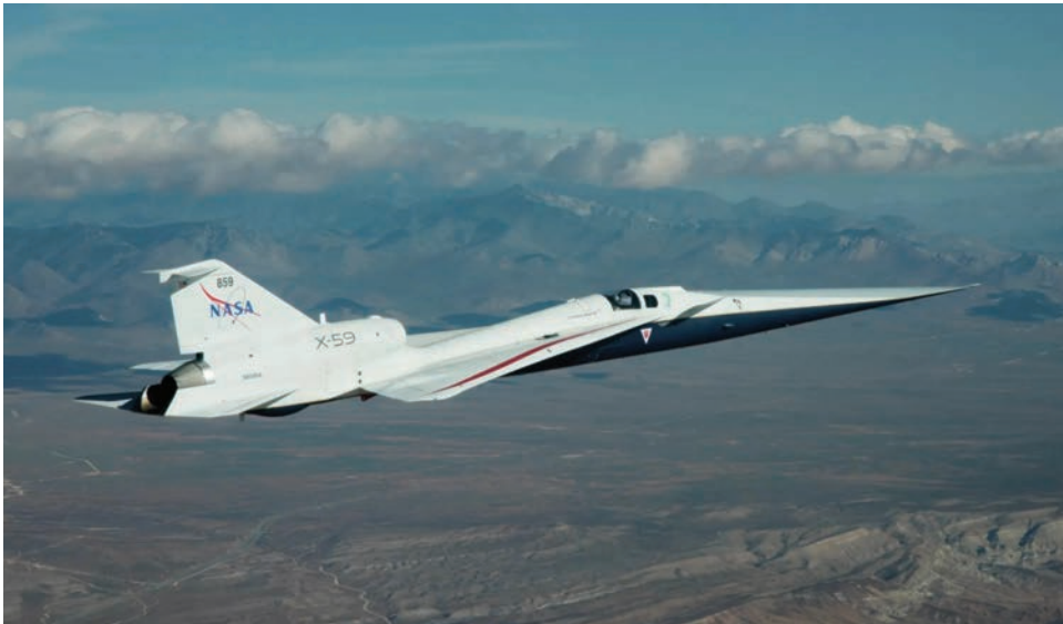
NASA's Low Boom Flight Demonstrator program, which oversees the development and testing of the X-59 experimental supersonic aircraft, aims to soften the sonic boom to a quieter "thump."
