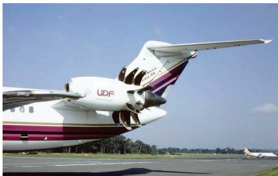
Research on unducted fans has a long history, including the GE 36 program, which ended in 1989.
