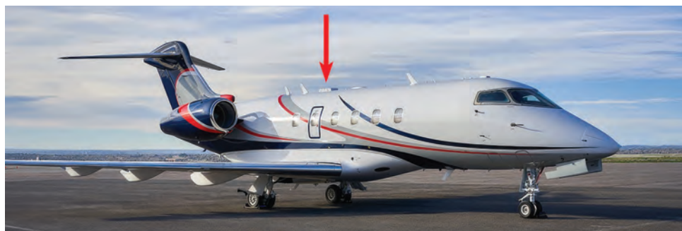
The Gogo Galileo small form-factor HDX antenna (arrowed) installed on a business jet, enabling Eutelsat's OneWeb LEO connectivity onboard. Credit: Gogo.
