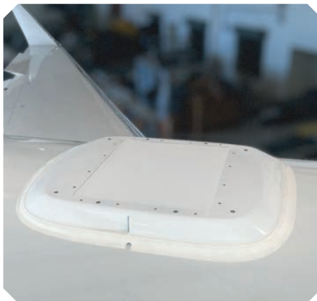
The Starlink electronically steered antenna mounts on the top of the fuselage.
