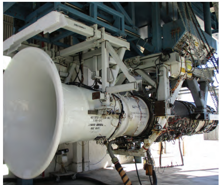
One of many dust ingestion tests for the RISE program, which are critical for understanding how this new engine architecture will function in harsher environments.
