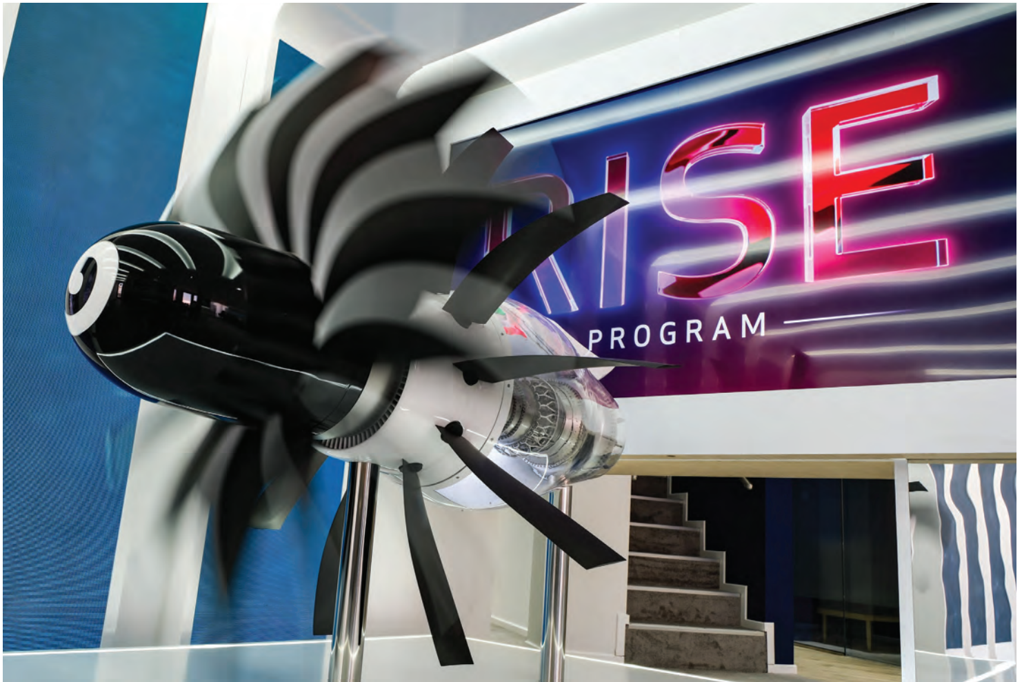
A model of the RISE program's Open Fan demonstration engine, which is aiming for 20% better fuel efficiency and improved durability.
