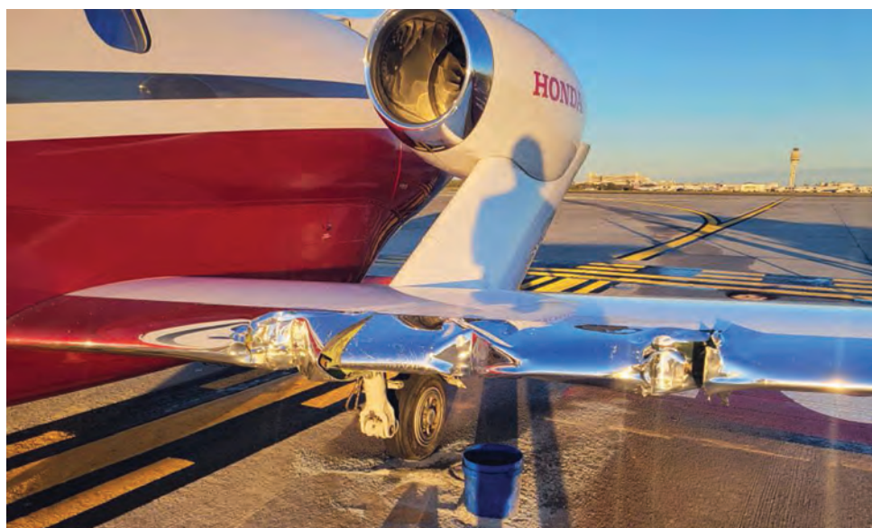
An exceedance of the published crosswind component was a likely factor in a runway excursion at Orlando International Airport that damaged this HondaJet's left wing and spar.
