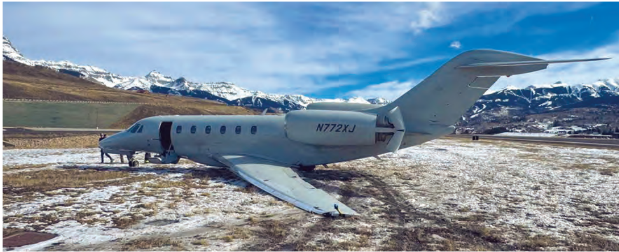
This Citation X landed at Telluride, Colorado, after encountering gusty, variable winds during the approach and touchdown, leading to a runway overrun.
