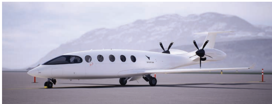
First flight of the Alice electric aircraft is expected by the end of the year, using the reconfigured version with engines mounted on the aft fuselage instead of the wingtips.
