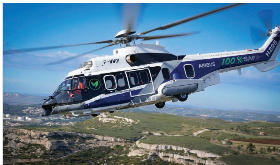
The Airbus H225 test helicopter flew with an unblended SAF derived from used cooking oil provided by TotalEnergies.
