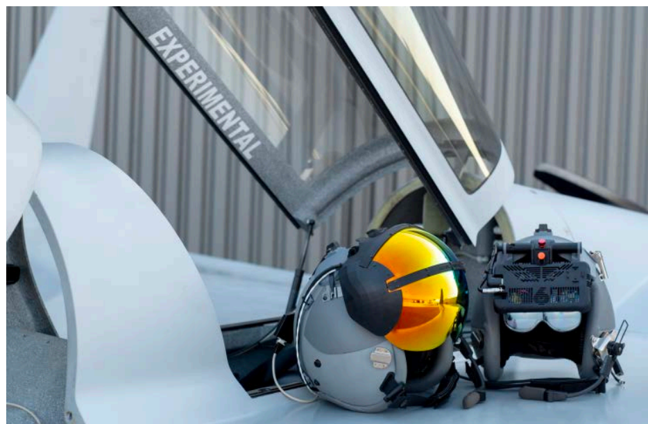
Red 6 uses a specially equipped helmet to let pilots see an augmented reality 3D virtual asset for training. It is working toward a 150-degree field of view.
