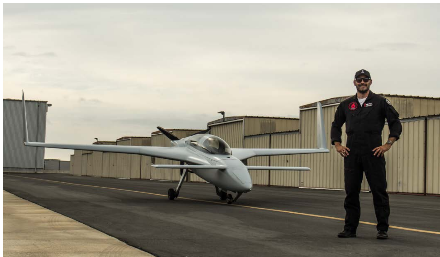
Dan Robinson built a Berkut composite, canard-configured experimental amateur-built airplane that now serves as the flight-test platform for the Airborne Tactical Augmented Reality System (A-TARS).
