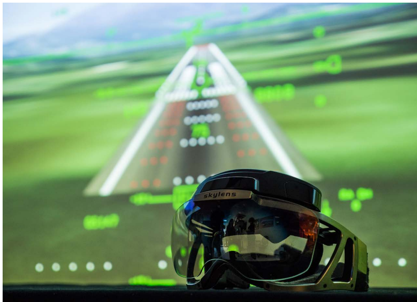
The Universal Avionics SkyLens HUD allows pilots to make FMS selections by using the HUD to look at a waypoint, airport, or navaid and then choose that using a selector button or manipulating the system via voice commands.
