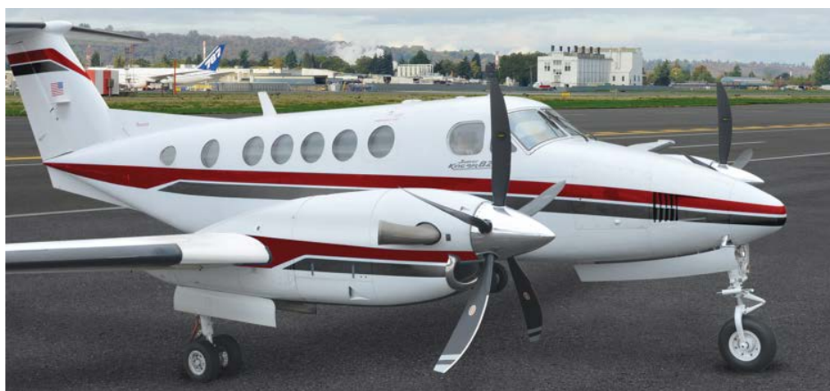
Hartzell says its new composite five-blade swept propeller for King Air 200-series aircraft weighs 48 pounds less than OEM-installed propellers.
