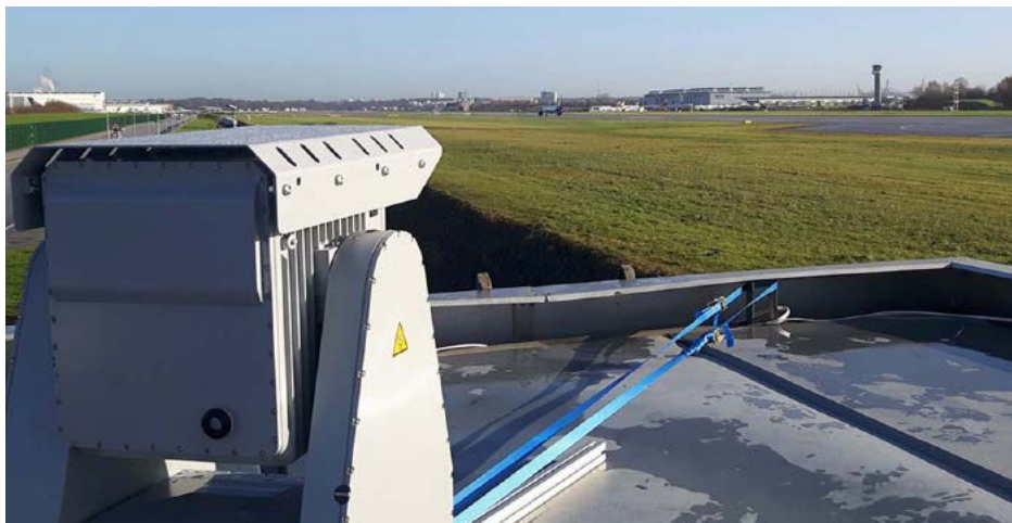
Hensoldt's Xpeller system can detect UAVs from several miles away.
