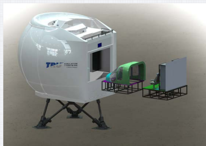
TRU Simulation's Odyssey H sim employs a roll-on/roll-off cockpit configuration to allow training for different helicopters in one sim.
