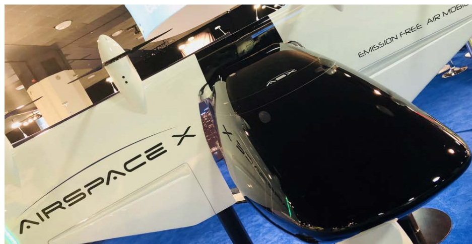
AirSpaceX’s Mobi-One eVTOL is designed to autonomously take off like a helicopter, fly like an airplane, and transport passengers or cargo between urban centers, suburbs, and airports within 60 miles at speeds up to 250 mph.
