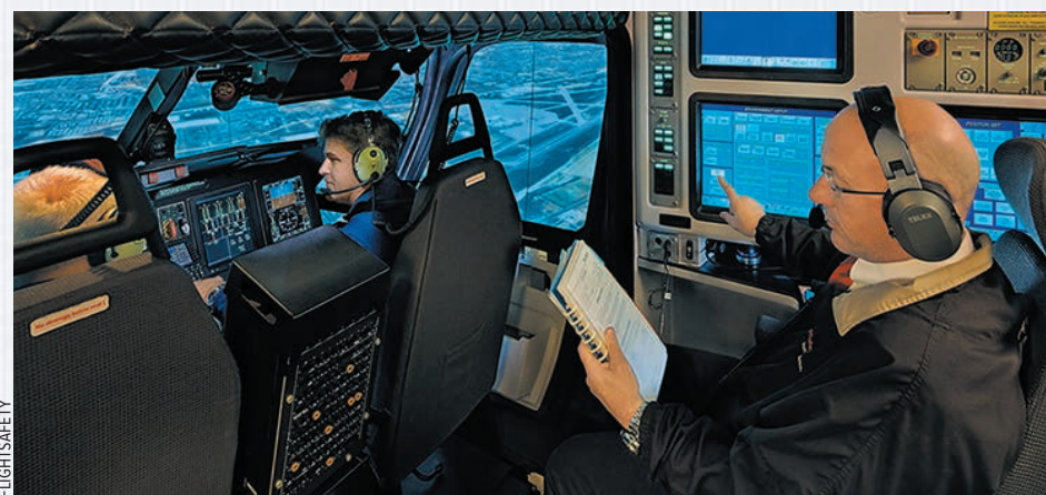
FlightSafety's level-D sims like this Sikorsky S-76D use a glass mirror display for brighter and sharper images.
