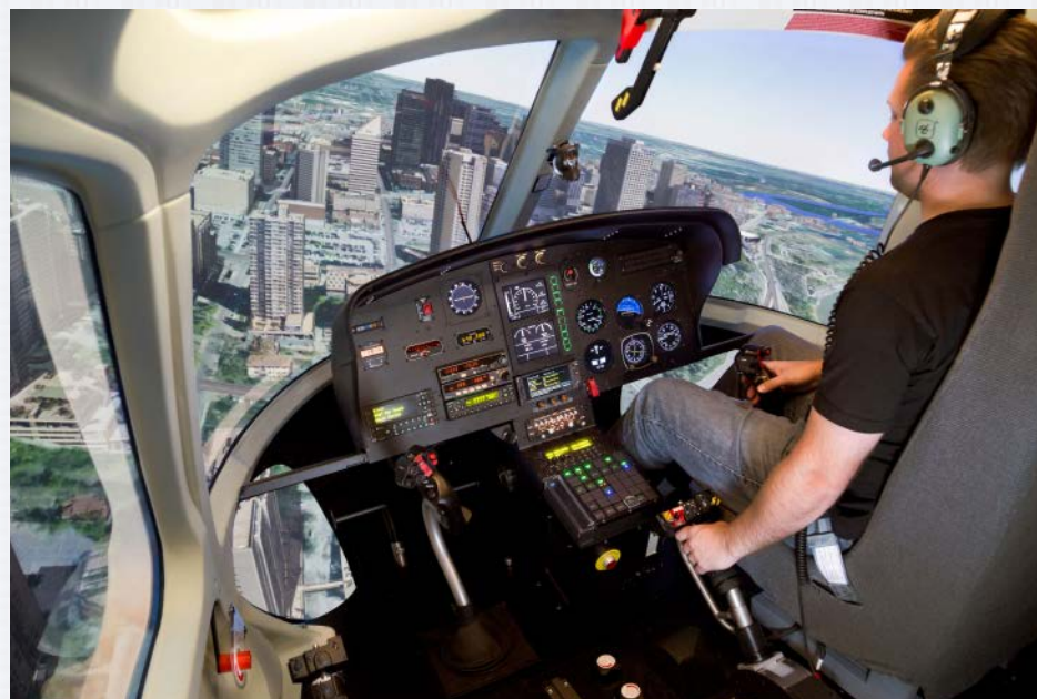
Frasca's small-stroke Motion Cueing System allows pilots to adapt faster to fixed flight training devices like this Airbus H-125 sim.
