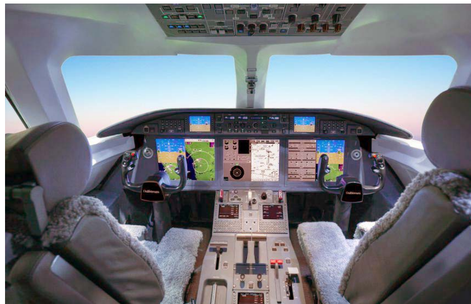
The Gulfstream PlaneView280 flight deck features three 15-inch displays and unique standby multifunction controllers that double as standby displays.
