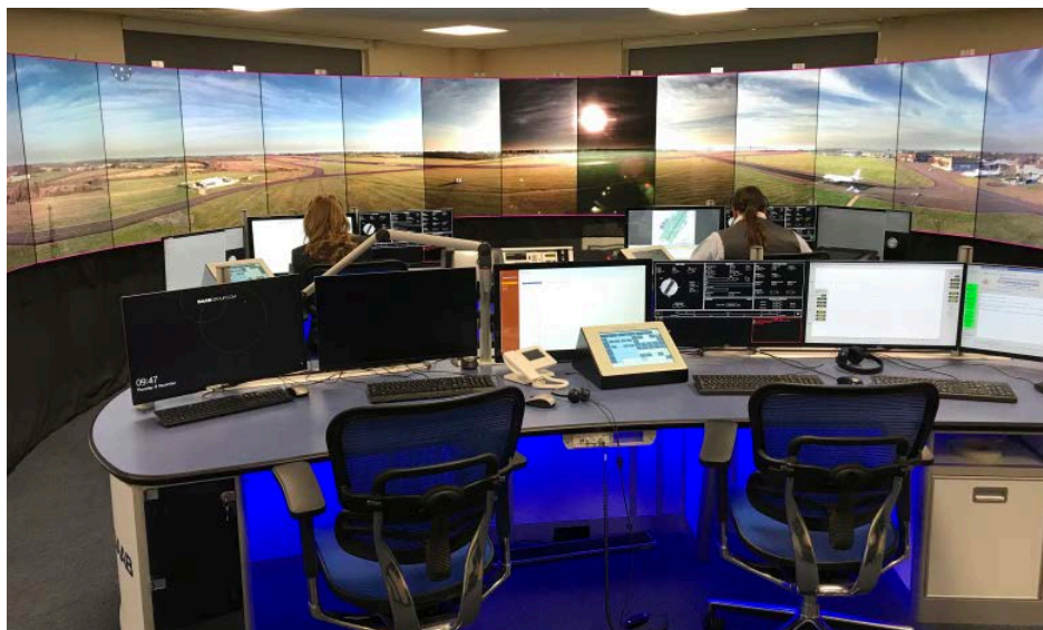
The Cranfield digital control center presents a 360-degree view of the airfield and its environs. Note the dimming applied to two screens in the center to minimize the glare from the low winter sun.
