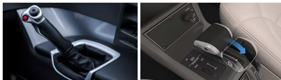
Recognizing that many operators fly without the rearmost three seats, Cirrus added wider center seats. For the pilot the sidestick falls readily to hand, as does the new autothrottle.
