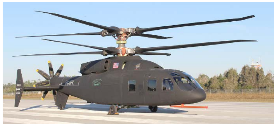
The SB>1 Defiant employs a rigid coaxial main rotor with an eight-blade pusher propeller.
