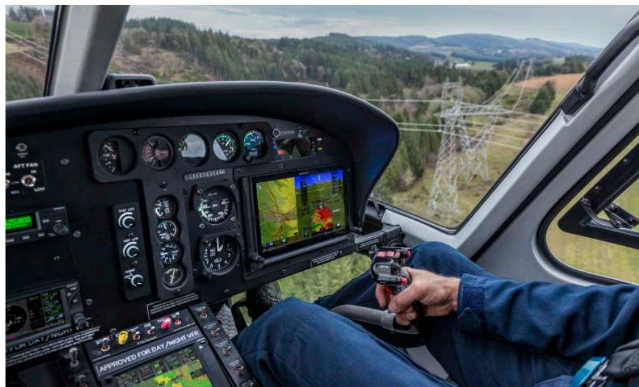
Garmin's touchscreen TXi displays for helicopters include knobs for alternate inputs.
