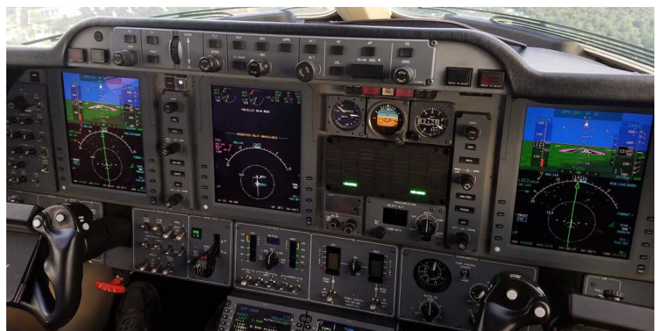
Winner Aviation installed this Collins Aerospace Pro Line 21 airspace modernization package on a Hawker Premier I. It will prepare the aircraft for the 2020 ADS-B mandate and beyond.
