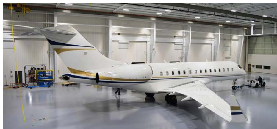
This Bombardier Global Express XRS launched the service entry of Duncan Aviation's new maintenance facility at Utah's Provo Municipal Airport last month. The long range twinjet will receive a 120-month airframe inspection and 10-year landing gear overhaul during its stay.
