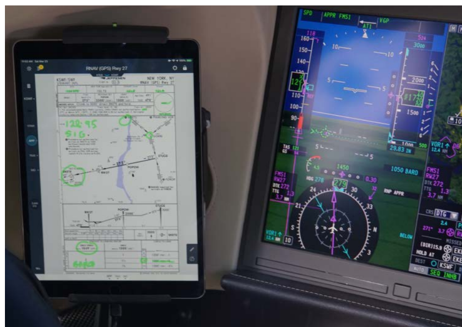
Jeppesen's Mobile FliteDeck is still popular among professional pilots, shown here with an annotated approach plate on an iPad mounted in a Bombardier Global 7500.
