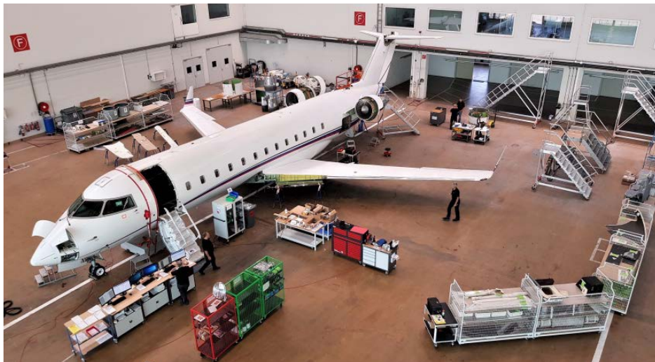
Nomad Technics completed an ADS-B Out installation on this Maltese-registered Bombardier Challenger 850 during its six- and 12-month inspection.
