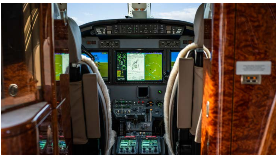
Stevens Aerospace and Defense recently completed its first installation of a Garmin G5000 avionics suite in a Citation XLS, along with fresh paint and interior. (Photo: Stevens)
