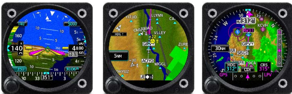
Garmin's GI 275 displays offer touchscreen and dual-concentric knob interfaces. Shown here are an attitude indicator (left), multifunction display (center), and HSI with map (right).
