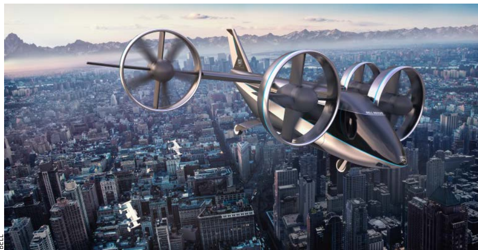
The four-rotor version of Bell's Nexus could be all-electric- or hybrid-electric-powered.
