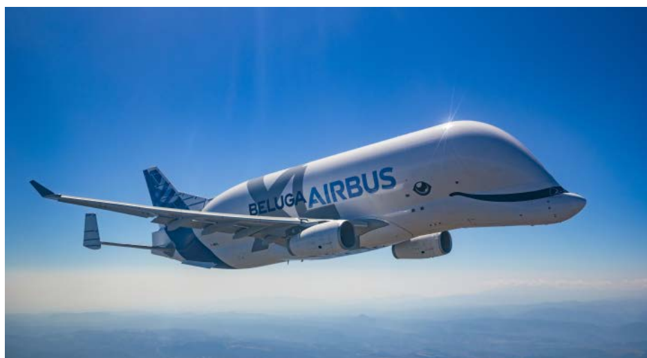
The Airbus Beluga XL can carry 30 percent more cargo, by volume, than its predecessor and fly to a range of 2,200 nm.
