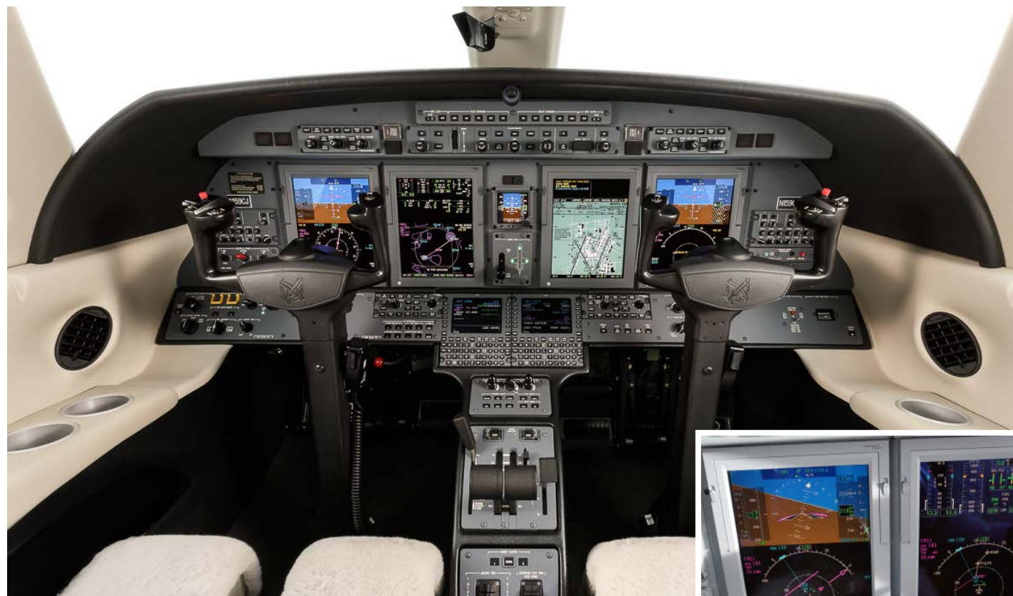
The Collins Pro Line 21-equipped CJ4 flown for this report was equipped with the optional second FMS. Dual cupholders for each pilot add a convenience to the CJ4's flight deck.
