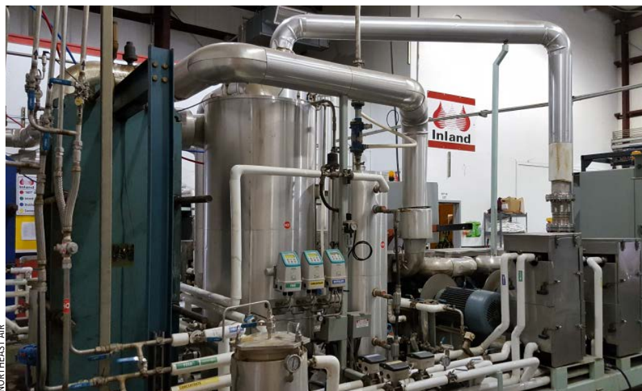
Inland's facility at PWM can distill approximately 10,000 gallons of pure glycol a week and can blend up to 50,000 gallons a day of Type I ADF in case of extended storms. Portland International Jetport is the first airport in the U.S. to rely solely on recycled deicing fluid.
