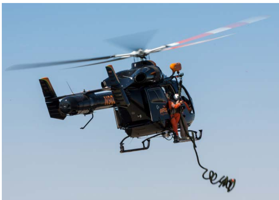
The MD Helicopters MD902 employs the Notar system as a way to avoid LTE.
