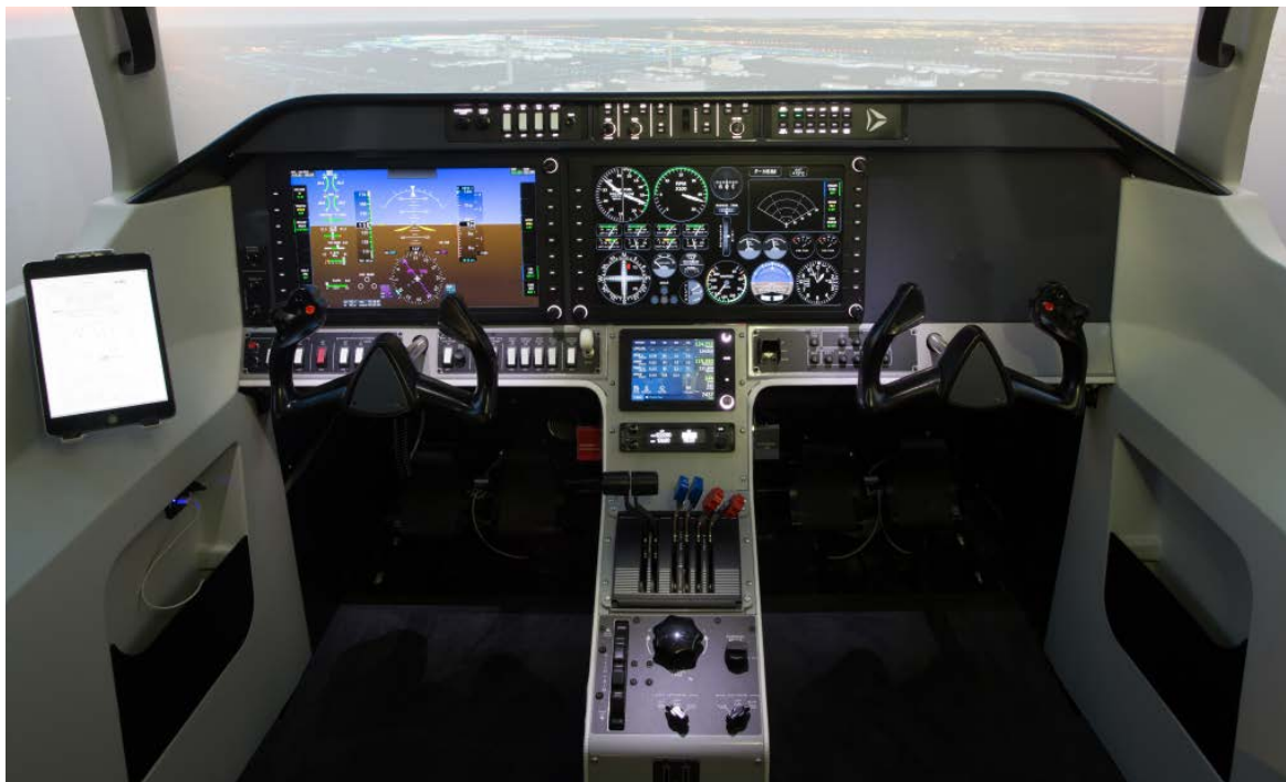
The Alsim AL250 is a generic sim that can be modified to replicate the cockpits of typical single- and twin-engine airplane models.
