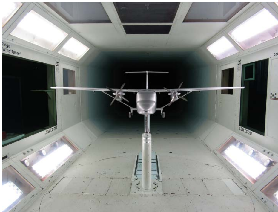
The wind-tunnel model of the Cessna SkyCourier was fitted with electric motors and scaled propellers calibrated to represent the thrust produced by the real aircraft.
