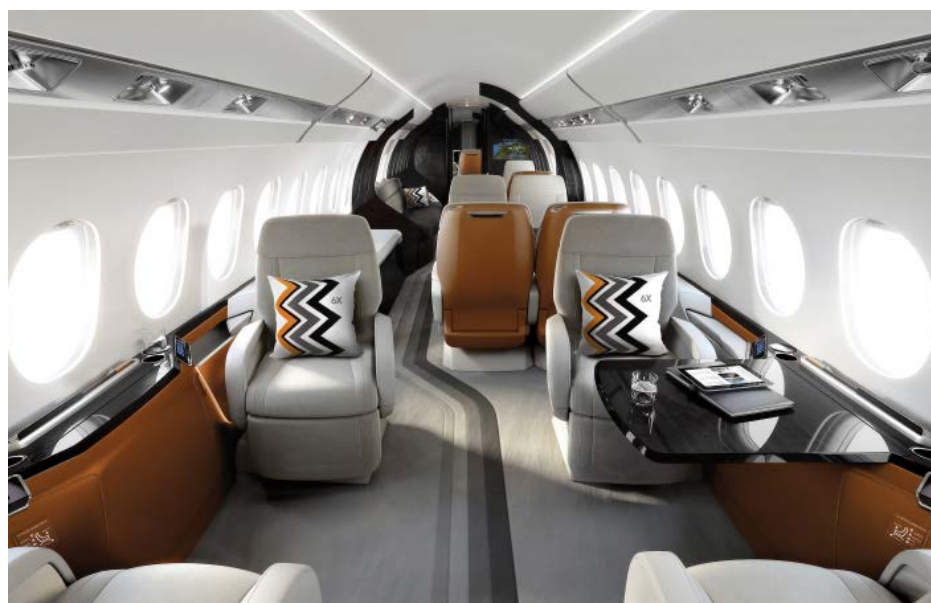
The cabin of the Falcon 6X will be 6.5 feet high and 8.5 feet wide, which Dassault says is “the highest and widest cross section in a purpose-built business jet.” At nearly 40.4 feet long, it is more than 20 inches longer than the cabin of the Falcon 5X.
