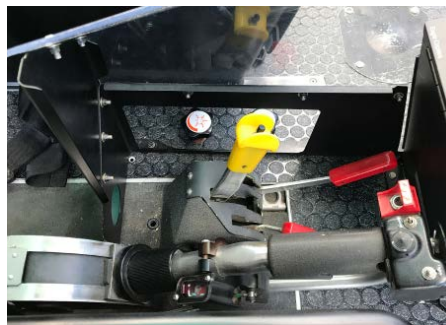
In the accident helicopter, the fuel-cutoff switch is on the floor next to the collective..
