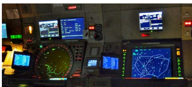
As part of the FAA's NextGen program, air traffic control towers and Traccon facilities are transitioning from the old ARTS IIE analog flight-tracking systems (left) to fully digital STARS Elite systems (right).
