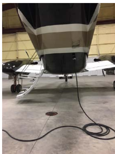
On the ground, Peter Schiff Aero's electric air-conditioning system in the King Air runs off a 220-volt extension cord plugged into a receptacle in the aft lower fuselage.
