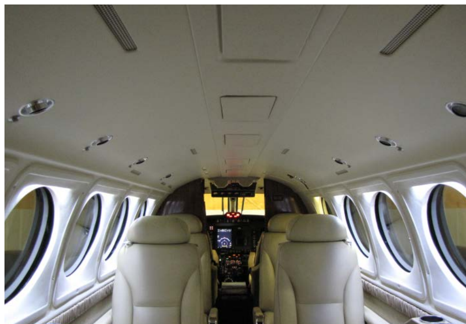
The Peter Schiff Aero electric air-conditioning system installed by Hampton Aviation in the company's King Air 200 delivers chilled air from overhead heat exchanger vents.
