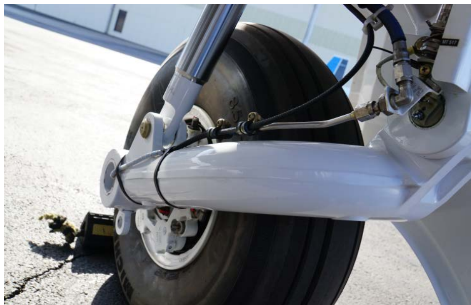
Advent Aircraft's eABS anti-skid braking system on the PC-12 adds a new wire harness, connecting the wheel speed sensor to the system's electronics.
