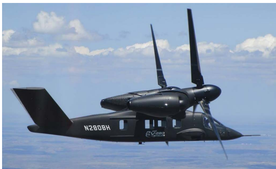
Bell's V-280 Valor refines the V-22 Osprey tiltrotor concept by introducing tilting blades, rather than the whole nacelle rotating.
