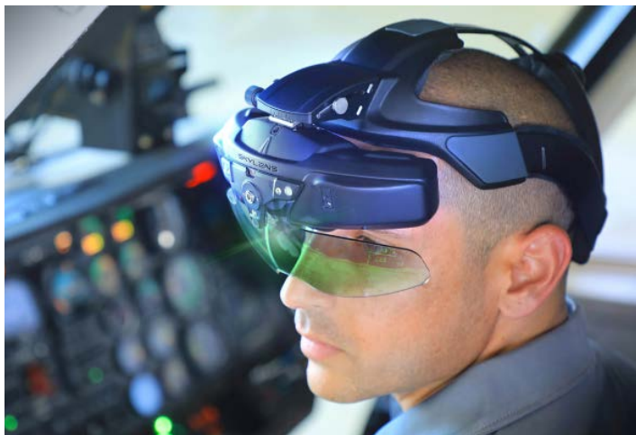
EASA has approved Universal's ClearVision system with SkyLens head-wearable display on the ATR 72/42.
