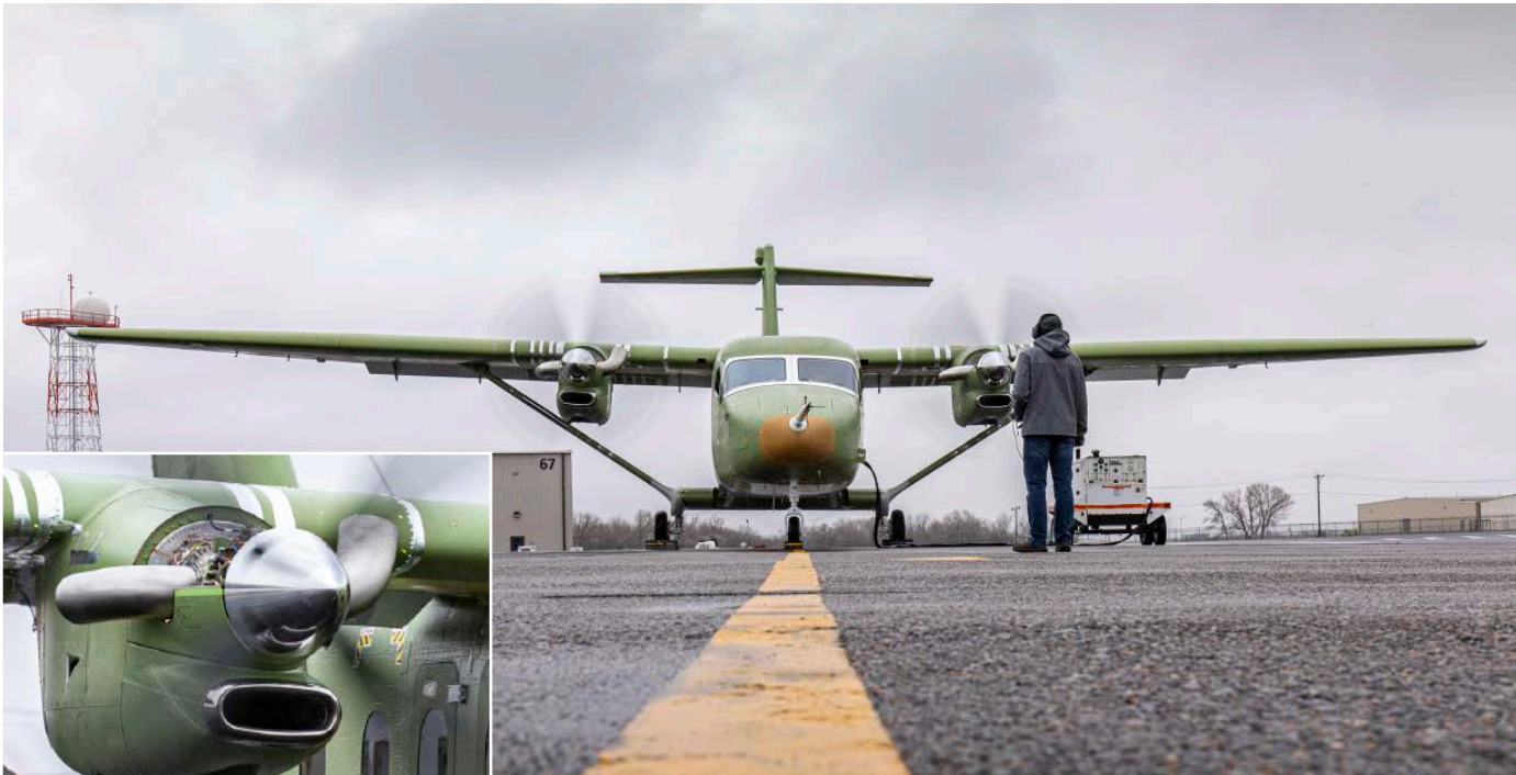
Textron Aviation has successfully completed initial ground engine tests of the Cessna SkyCourier's two Pratt & Whitney Canada PT6A-65SC turboprop engines (inset close-up). FedEx is the launch customer for the utility twin, with a firm order for 50 and options for 50 more.
