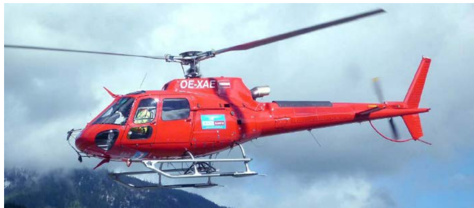
BLR Aerospace's FastFin enhancement includes vortex generators and tailboom modifications to improve anti-torque characteristics in low-speed and hover operations.
