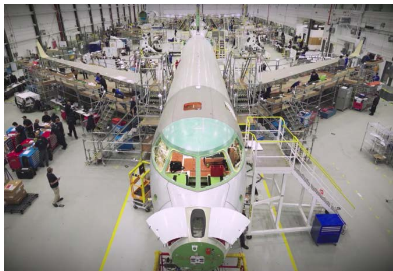
The fifth flight-test Global 7000, currently on the production line, has already been outfitted with the new lighter, and final, version of the wing for the ultra-long-range jet.
