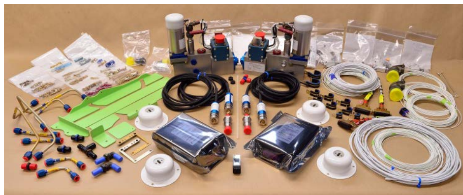
Advent recently received certification for the eABS braking system on the King Air B300. The company also offers the system on the Eclipse and Pilatus PC-12.
