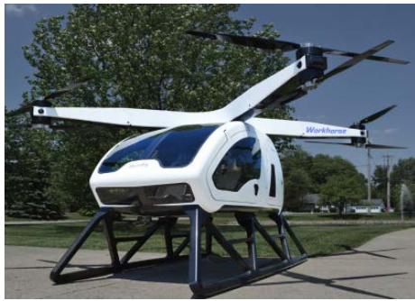
The eVTOL SureFly electric helicopter offers redundant electrical supply thanks to an onboard generator.
