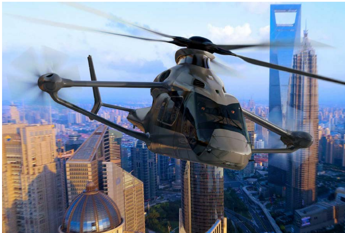
Airbus Helicopters' high-speed concept rotorcraft, dubbed Racer (for rapid and cost-effective rotorcraft), will have a main rotor, two lateral pusher rotors and a joined "box wing" configuration. Racer will cruise at 220 knots, although it will be able to fly at higher speeds.
