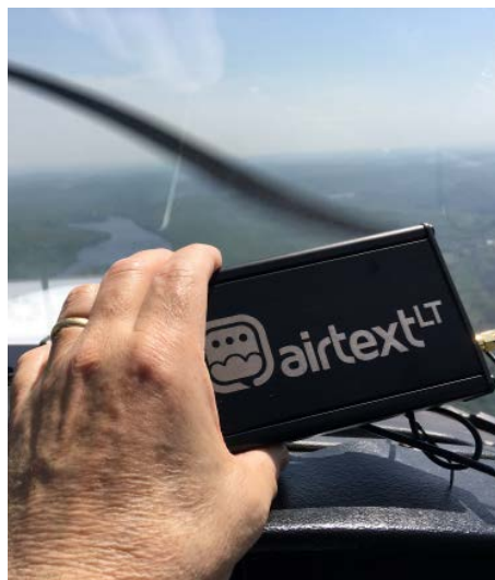
The portable Airtext LT offers text-only capability to make satcom affordable to operators of smaller aircraft.
