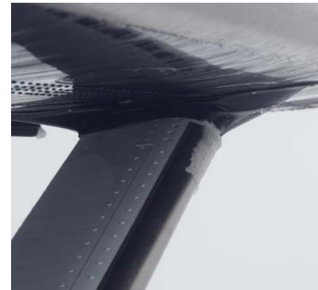
The Kodiak is at home in mountains and in known icing conditions, and the TKS system helps prevent ice accumulation, but can also serve to remove existing ice.
