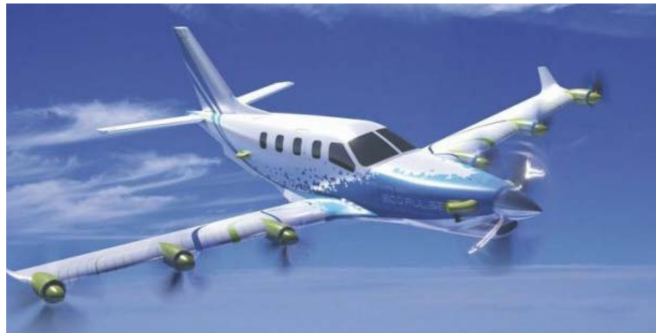
Daher, Safran, and Airbus will join forces to create EcoPulse, a wing-mounted distributed hybrid-propulsion demonstrator based on Daher's TBM platform. First flight is expected in 2022.
