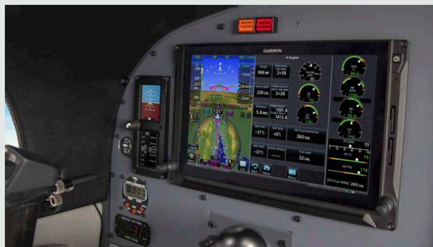
Garmin's EIS TXi display can now serve as a replacement for old engine gauges on certain PT6A-powered single-engine turboprops.
