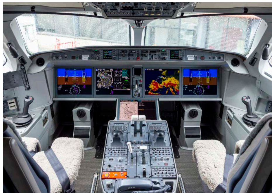
The Airbus A220 flight deck features a five-panel Collins Pro Line Fusion avionics suite and sidestick fly-by-wire controls.
