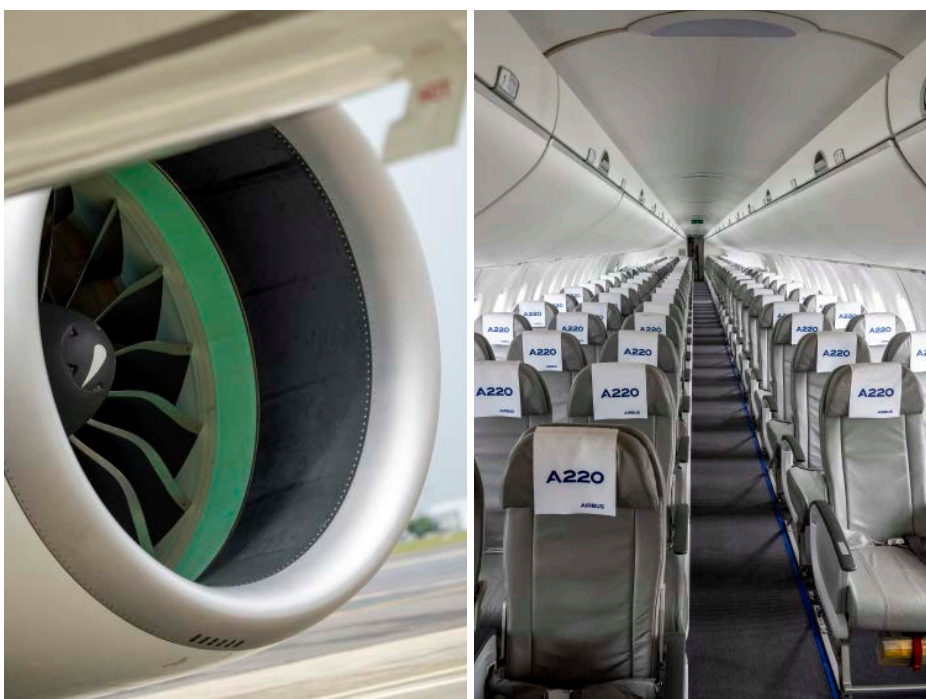
The left nacelle and P&W PW1000G geared turbofan. On the inside, the demonstrator has a two-plus-three seating arrangement, with extra-wide center seats in the three-seat rows.
