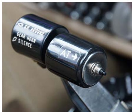
The autothrottle disengage button is located on the right power lever.
