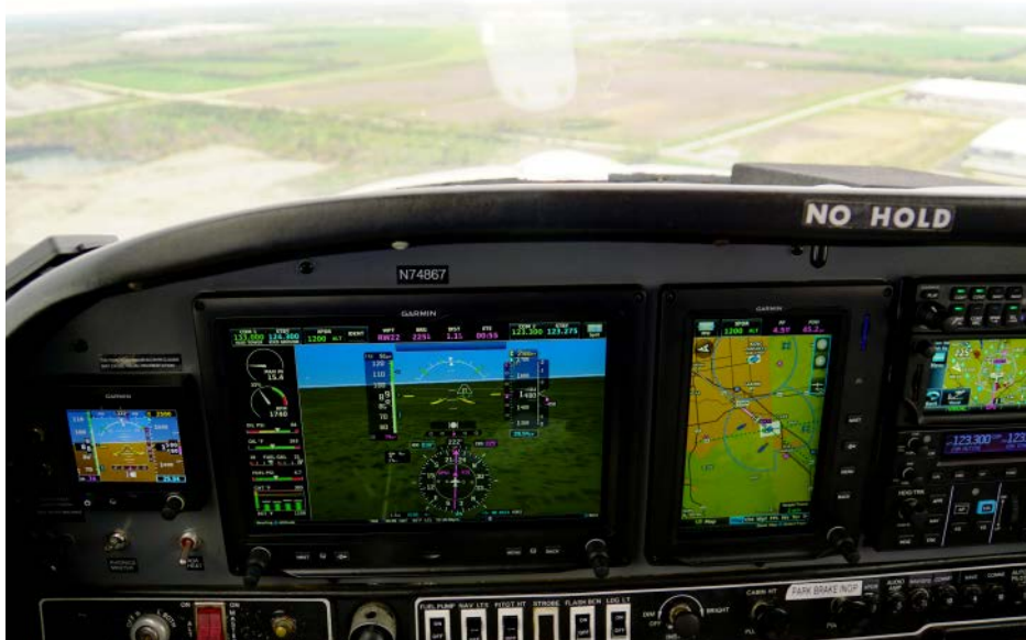
The focal point of the Grumman Tiger A1N flew in was its two G3X Touch units, a 10.6-inch GDU 460 in landscape orientation and a 7-inch GDU 470 in portrait mode.
