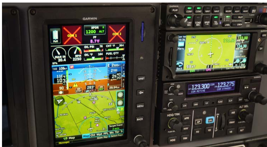
Garmin's 7-inch G3X Touch can act as a full backup with PFD, MFD, and engine information as well as the ability to continue working with the GFC 500 autopilot after a main display failure.
