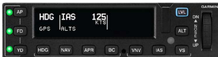
The Garmin autopilots are designed to interface with G500/600 displays.
