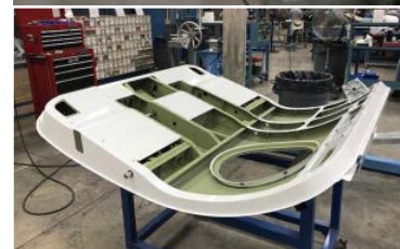
Cessna is making progress on assembling large sections of the Denali, such as the cargo door, and aft cabin lower quarter panel, above.
