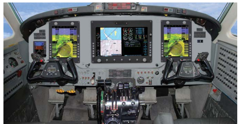
The King Air NextGen flight deck includes new PFDs and MFD.
