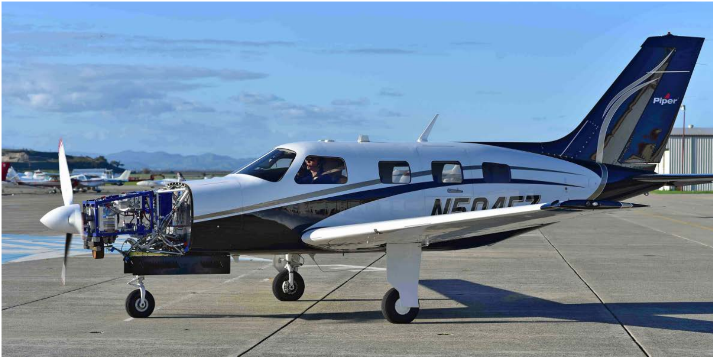
Clean energy start-up ZeroAvia started flight testing its hydrogen fuel powertrain system on a Piper M350 piston single, but it plans to offer the technology to regional aircraft operators by 2022.
