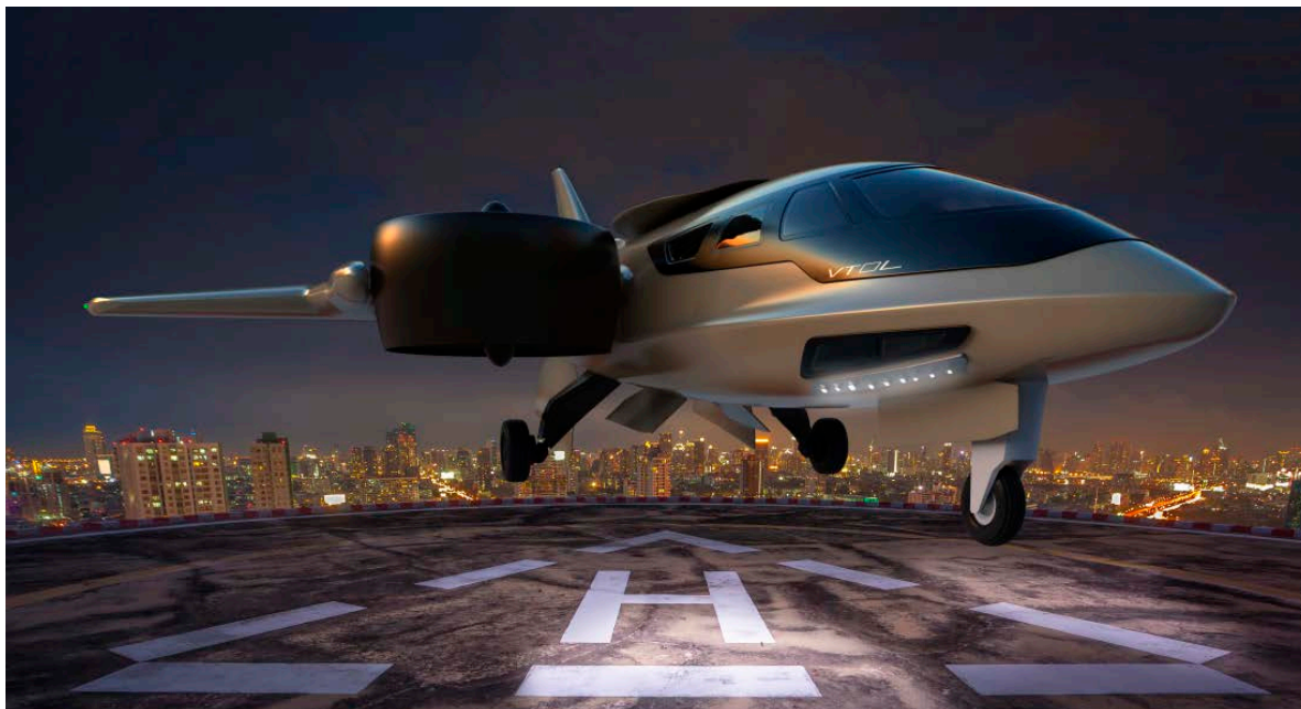
XTI Aircraft says the TriFan 600 hybrid-electric VTOL will have the speed, range, and comfort of a business jet and the ability to take off and land vertically using three ducted fans.
