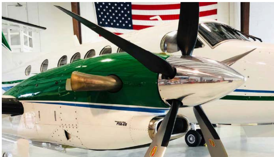
The most visible improvement in Blackhawk Aerospace's newly certified XP67A upgrade for the King Air 300 is the replacement of the four-blade Hartzell propellers with five-blade versions. Under the cowlings, the company swapped out the stock PT6A-60A engines with new updated PT6A-67As.
