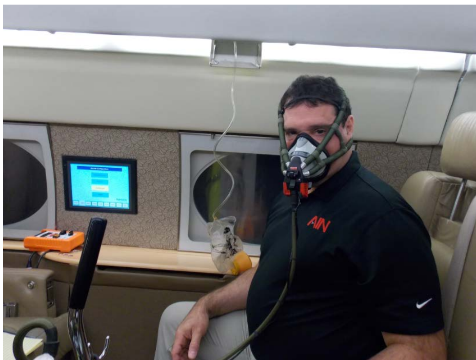
Part of the cabin-simulator curriculum is decompression training. The author wears a quick-don mask, usually worn by the copilot. It uses bottled oxygen to simulate breathing at altitude.
