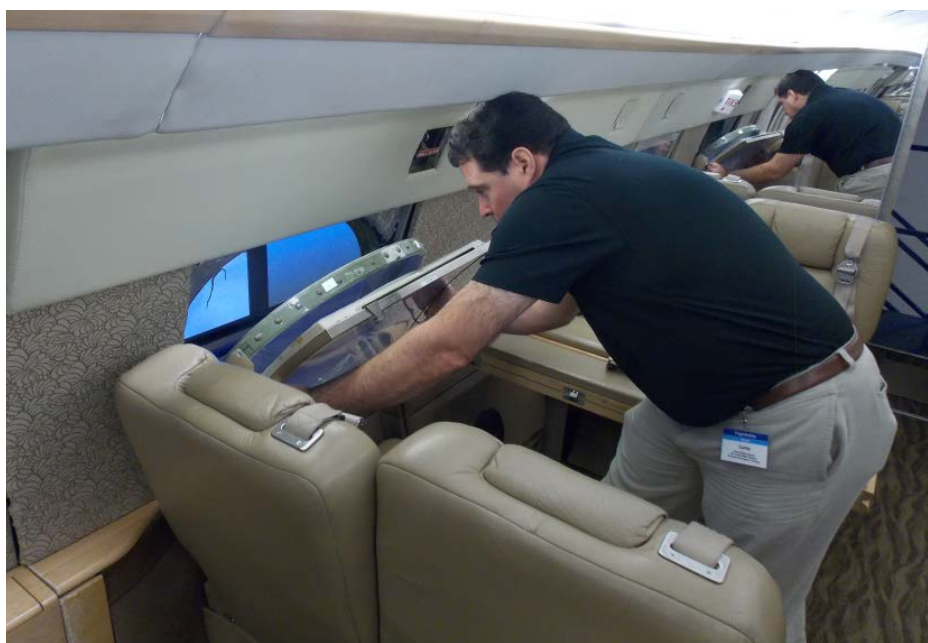
The cabin simulator is equipped with overwing exits that correspond to those on several types of business aircraft, and students learn to remove the windows to exit in an emergency.
