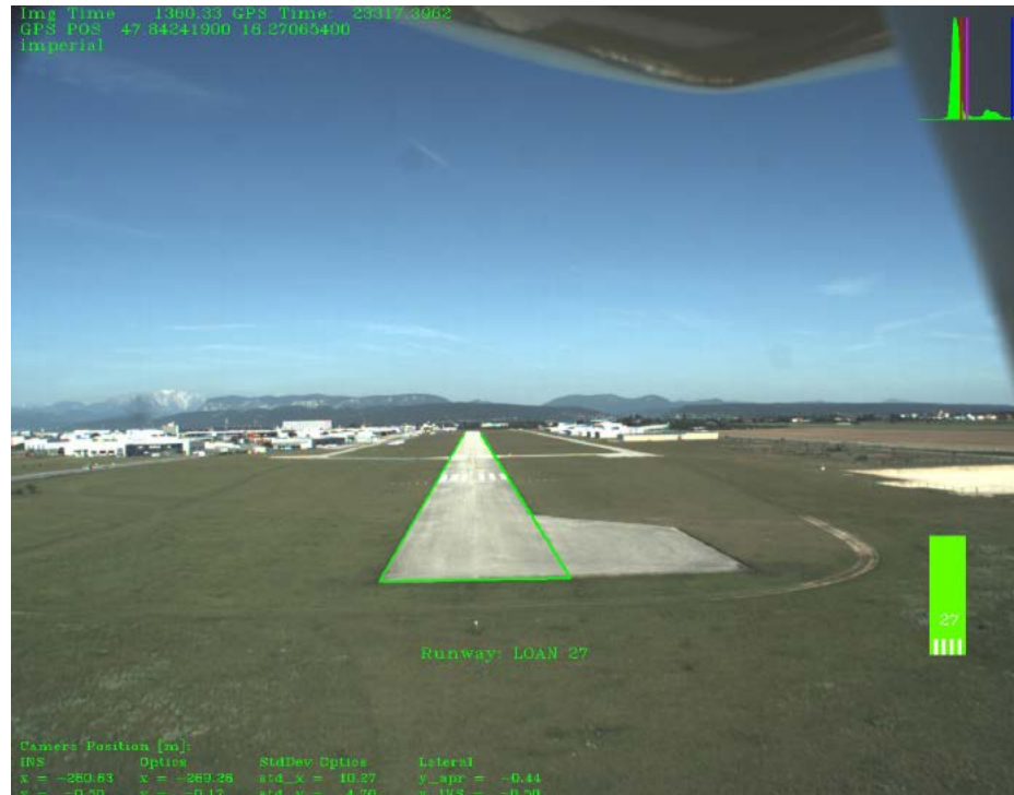
Vision-assisted navigation helped land a Diamond DA42 automatically, as part of a research project at the Technical University of Munich.
