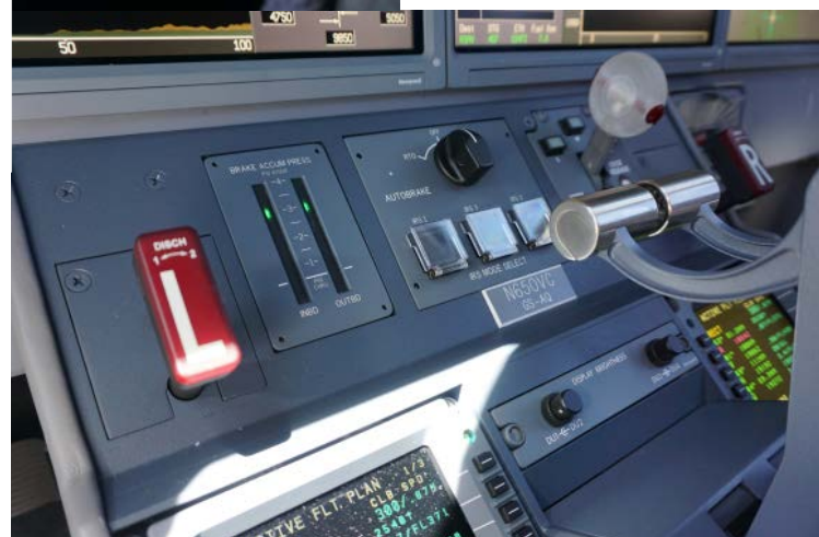
Top: Tony Briotta, demonstration pilot, flew left seat along with senior international captain Scott Curtis for the leg from Savannah, Ga., to Columbia, S.C. The new standby multifunction controller (bottom left) has a handy new utility page and opened up space to mount the autobrake controls on the tilt panel (right).
