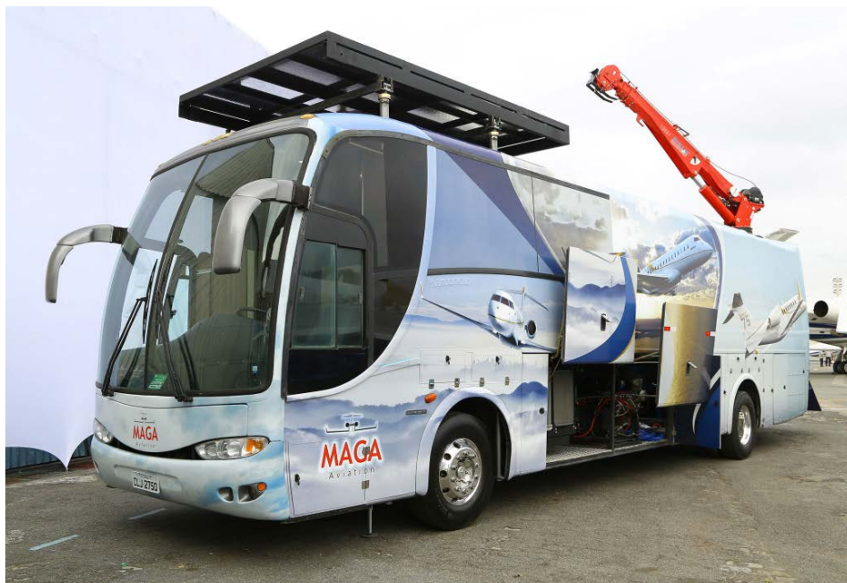
Newly authorized Bombardier Global service center MAGA Aviation introduced this mobile jet support vehicle at LABACE. It has a rooftop crane for engine removal, and a raised platform for working on jet tails.
