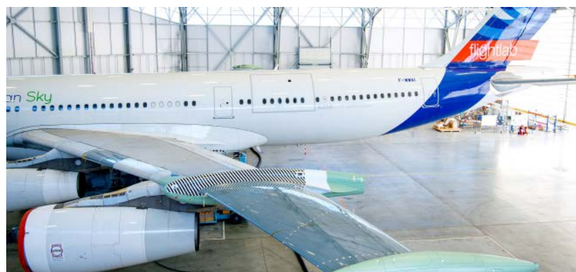
Airbus and partners in the Blade initiative are using the A340 prototype to test two wing designs that have the potential to yield significant fuel savings for airlines.
