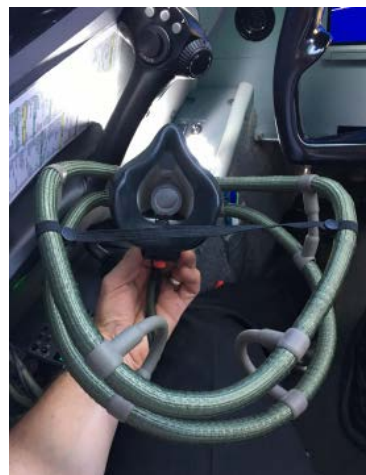
The design of oxygen masks makes them uncomfortable for use over several hours, as the rules require.
