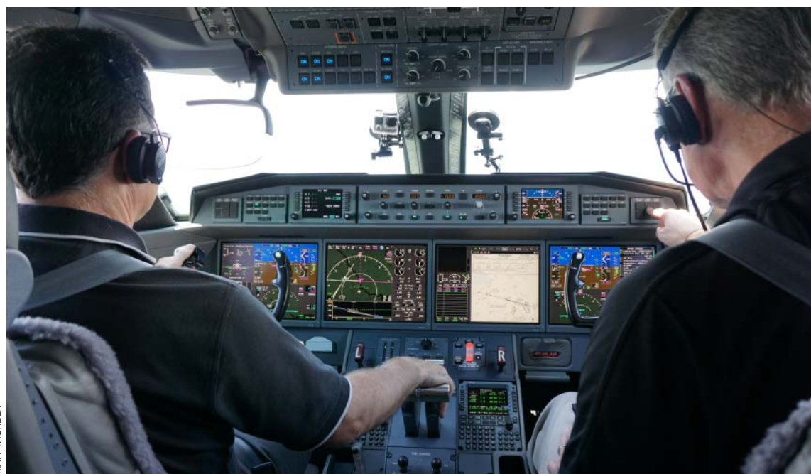
Top: Tony Briotta, demonstration pilot, flew left seat along with senior international captain Scott Curtis for the leg from Savannah, Ga., to Columbia, S.C. The new standby multifunction controller (bottom left) has a handy new utility page and opened up space to mount the autobrake controls on the tilt panel (right).
