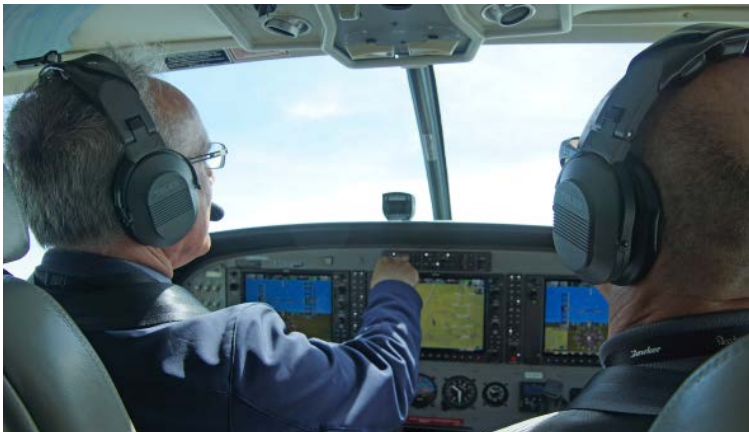
The newest versions of the Caravan EX are equipped with the Garmin G1000NXi, offering additional features compared with the G1000 on the airplane flown for this report.
