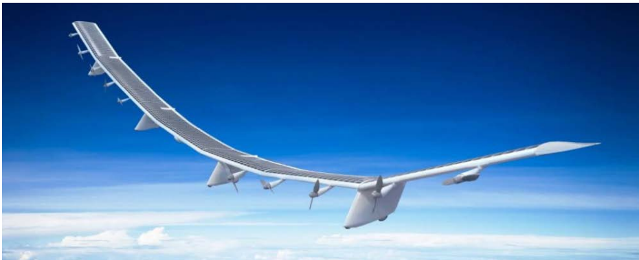
The Hawk30 solar-powered high-altitude platform system (HAPS) will serve as a stratospheric telecommunications solution that can stay airborne for months at a time.
