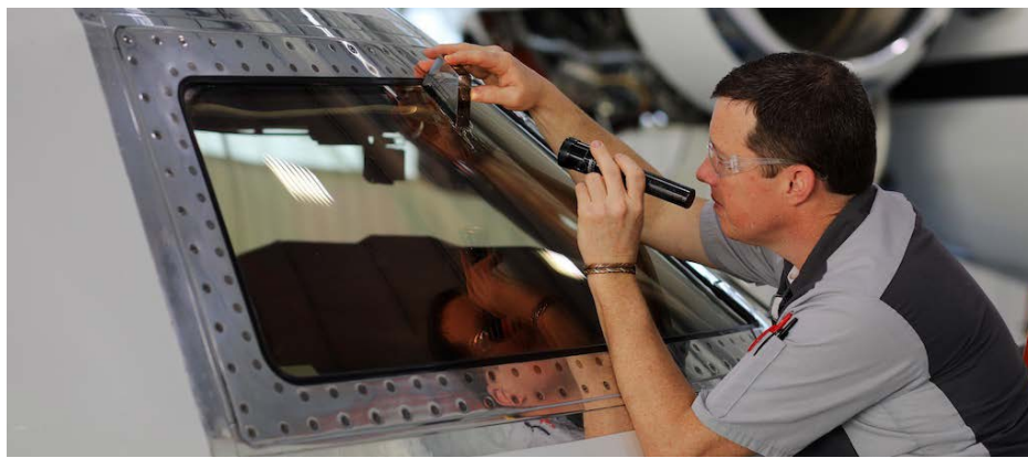
Duncan Aviation's non-destructive testing (NDT) services include eddy current, fluorescent penetrant, ultrasonic, and magnetic particle inspections on all aircraft makes and models.
