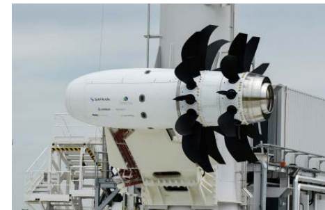
Safran has been running an open-rotor demonstrator at its facility in Istres, France, since May. The engine configuration could burn 15 percent less fuel than the CFM Leap.
