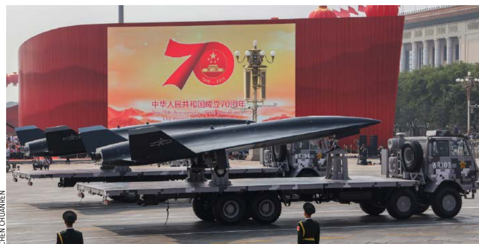
Two examples of the WZ-8 supersonic UAV were shown at a military parade on October 1. Note the pylon hooks and rocket motor exhausts.
