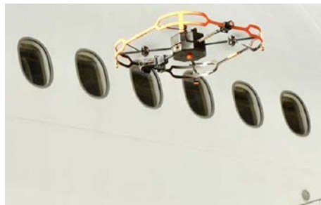
A Donecle drone used by AAR conducts an automated aircraft inspection.
