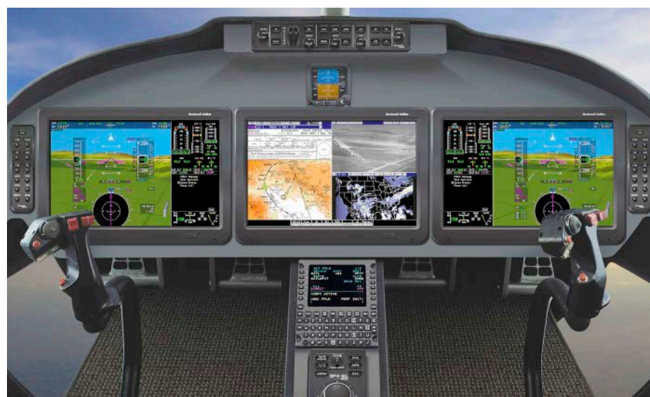
The touchscreen Collins Pro Line Fusion suite powers the AW609 flight deck.
