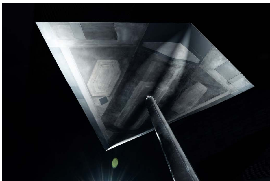
LOU includes doors for a weapons bay and landing gear. The thrust-vectoring nozzle is located above the rear part to shield it from ground-based sensors.
