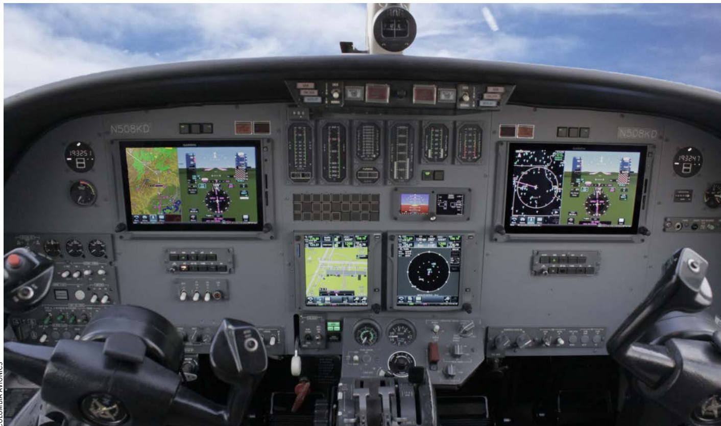
Columbia Avionics modernized this Citation 500's instrument panel with dual Garmin G700 TXi displays and GTN 750 com navigators.
