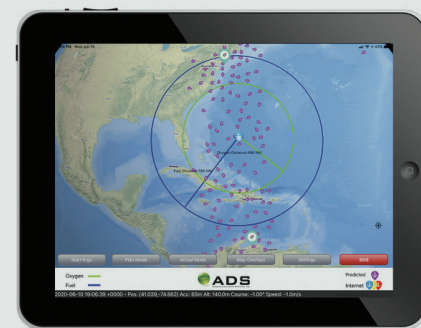
The Ergo 360 app displays fuel and oxygen range rings and shipping traffic, to help pilots deal with emergency situations in remote areas.
