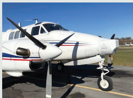
The Vu Cube passive millimeter wave sensor installed in the nose of an unpressurized King Air used for flight testing.
