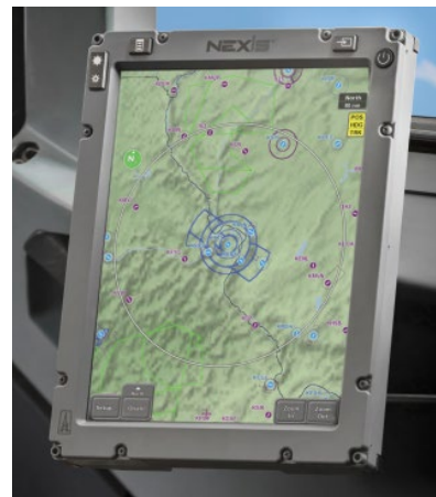
The Astronautics Nexis EFB adds modern touchscreen avionics to older cockpits.
