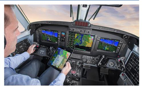
Garmin's G1000 NXi (next-generation) avionics suite, already certified in the King Air 200, adds faster processors, map overlays on the HSI and wireless connectivity to mobile devices via Garmin's Flight Stream 510.
