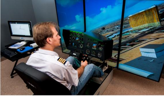
Today's graphics capability, with the widespread integration of GPS, allows manufacturers to give pilots a geospecific experience such as this Elite AS350 flying over the Las Vegas Strip.
