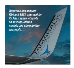
Other improvements for the Citation light jets include a 400-pound increase in zero-fuel weight, significant range increases, higher initial altitudes, a 12 to 15 percent boost in single-engine climb gradients, improved stability and extended wing life as a result of reduced fatigue.
