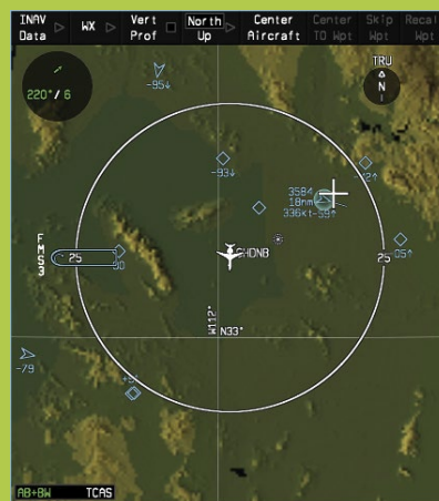
Honeywell’s implementation of the ADS-B IN cockpit display of traffic information.
