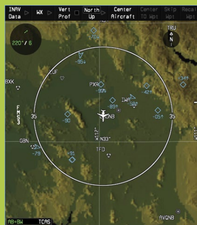
Honeywell’s implementation of the ADS-B IN cockpit display of traffic information.
