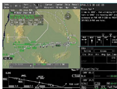
Above, IS&S is offering an autothrottle system to bring RNP approaches to PT6-powered aircraft. Honeywell's DynaCharts, below, populates displays with information from charts to ease workload. TopMax, right, brings HUD capability to smaller aircraft.
