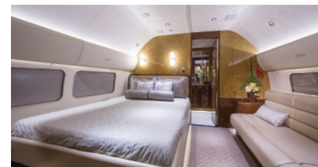
The adjustable bed in the VIP section of this BBJ, completed by BizJet, allows the passenger to maintain a level pitch regardless of the aircraft's attitude.
