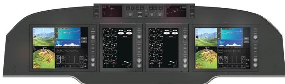
Avilon combines touchscreens with a minimal number of knobs and switches. Visual displays depict the state of the airplane on "tiles" that add up to a richly informative "main primary" display in front of each pilot. Each main primary is split into four of these tiles, essentially mini-displays adding up to a larger 12-inch display.
