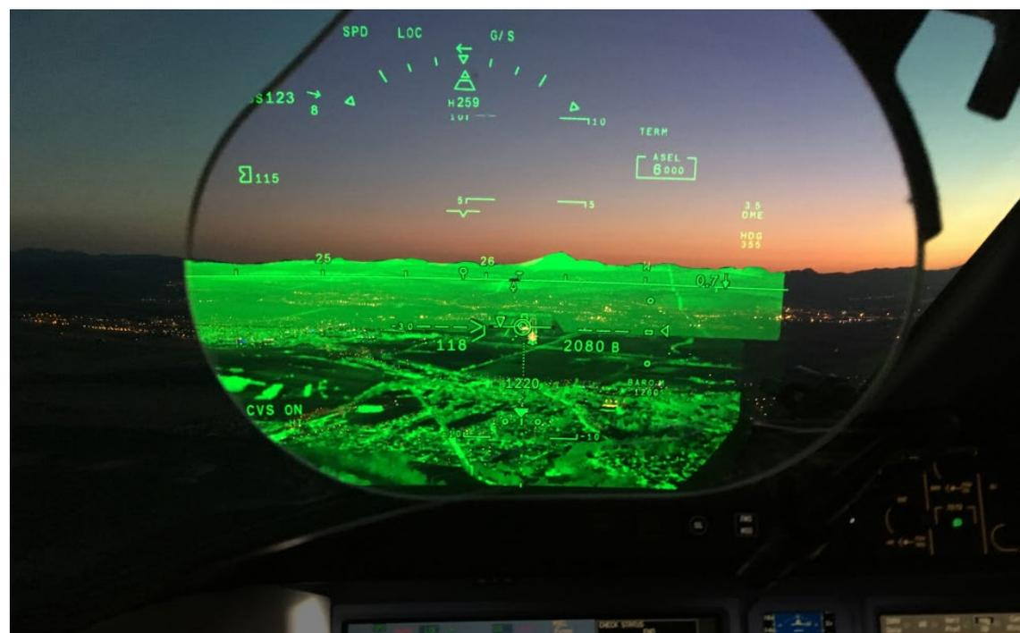
Effective March 13, pilots flying in the U.S. with an enhanced flight vision system such as Dassault’s FalconEye (pictured above), will be able to continue the approach to landing using only the images displayed by the EVS on the HUD, all the way to landing “in lieu of natural vision.”
