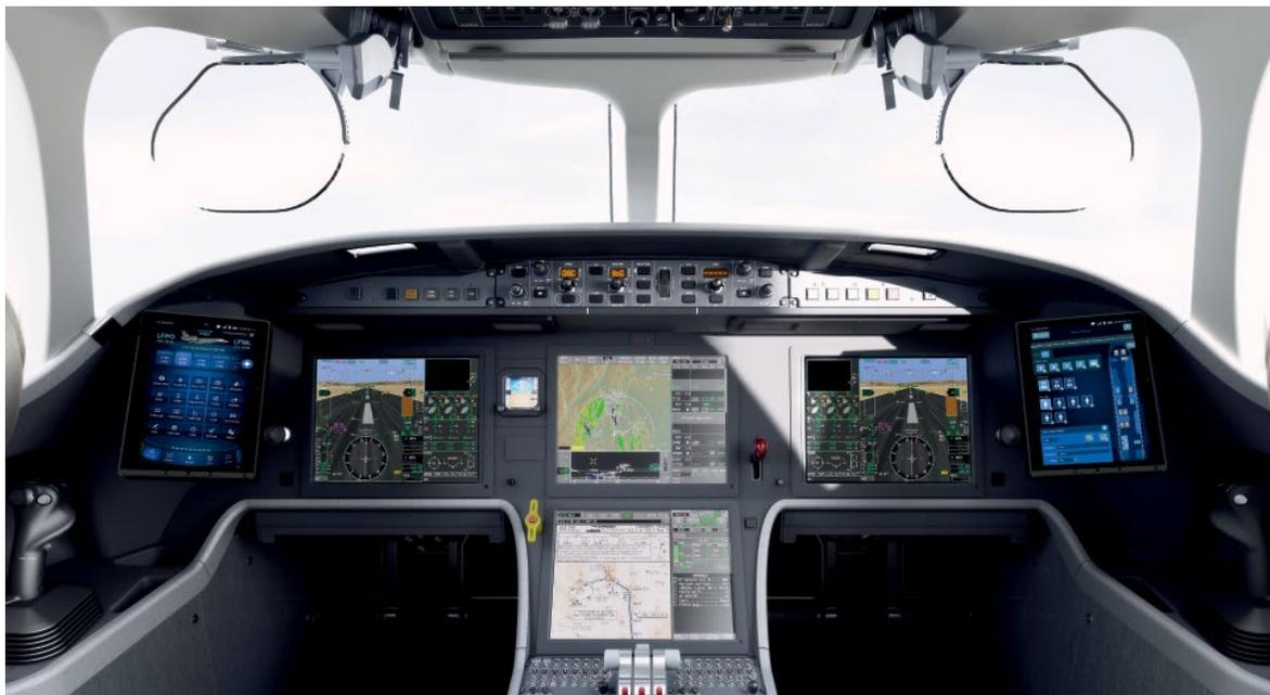
**Sidestick-operated fly-by-wire flight controls make for a clean, uncluttered flight deck. The 8X's EASy III avionics system, based on Honeywell's Primus Epic suite, features synthetic vision and 3-D digital radar. The FalconEye HUD and combined vision system is optional.**
