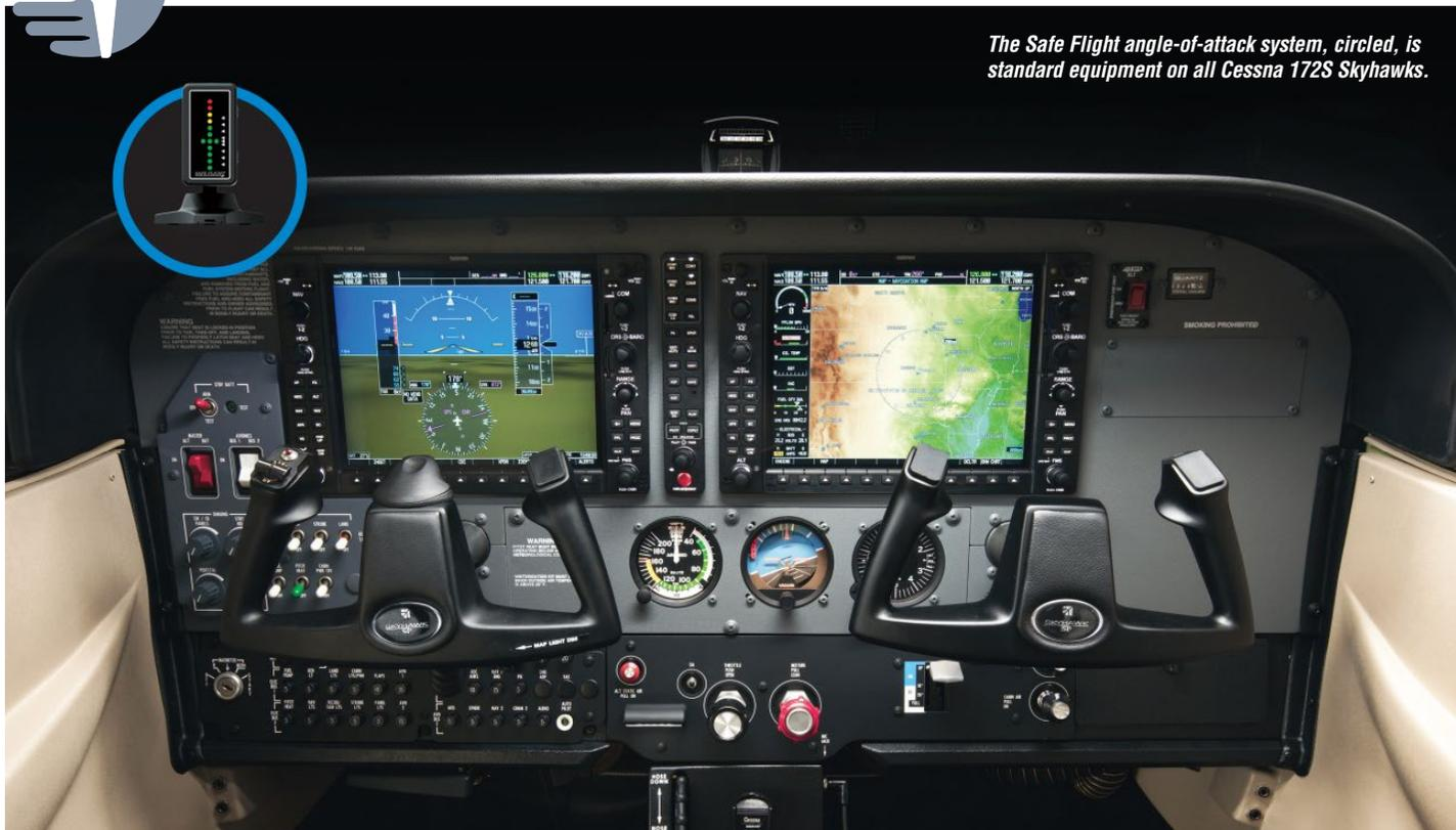
The Safe Flight angle-of-attack system, circled, is standard equipment on all Cessna 172S Skyhawks.
