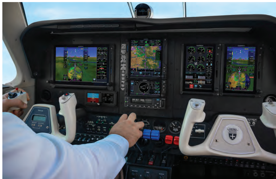
Garmin's Smart Rudder Bias automatically applies rudder to help when an engine fails in a piston twin, identifies the failed engine on the PFD, and applies Electronic Stability and Protection assistance, giving the pilot more time to deal with the emergency.
