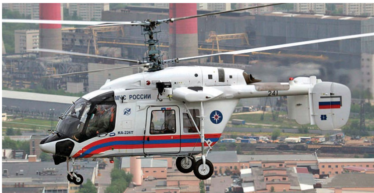
The Ka-226T, which has more power than its predecessor, has a maximum speed of 119 knots and a range of 270 nm.
