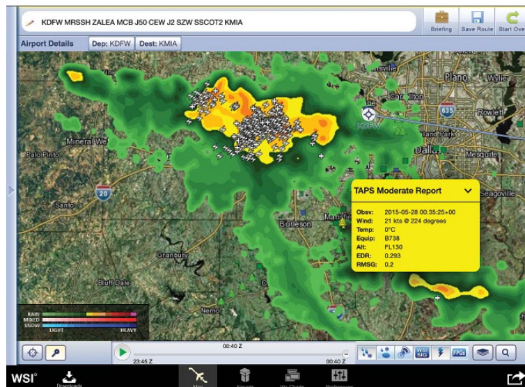
WSI's Pilotbrief will include turbulence information derived from the company's Turbulence Auto-Pirep System (Taps) installed in a number of airliners. Taps uses systems installed in the aircraft to measure turbulence beyond specified parameters.
