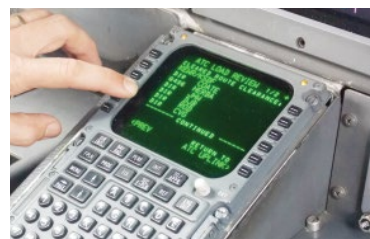
The DataComm system streamlines the departure reroute clearance procedure with new routing sent directly to the aircraft's flight management system.
