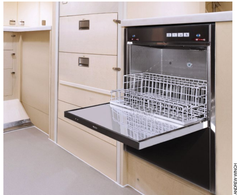
Jet Aviation Basel has developed for widebody aircraft a plug-and-play in-flight dishwasher with a three-minute wash cycle that runs on three liters of water.
